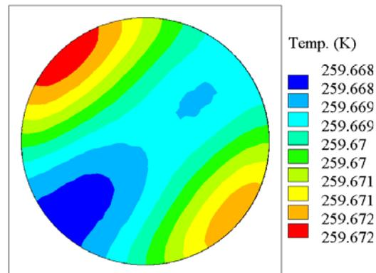
Figure 11. Temperature contours on surface of cold plate; ethanol as coolant.
