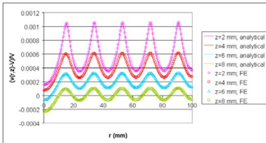
Figure 3. Comparison of analytical predictions to finite element predictions of the non-dimensional temperature in the meter plate.
