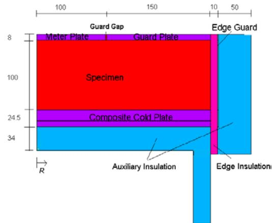
Figure 13. One quarter cross section of Guarded Hot plate for analyzing heat flow within the specimen; dimensions in mm.
