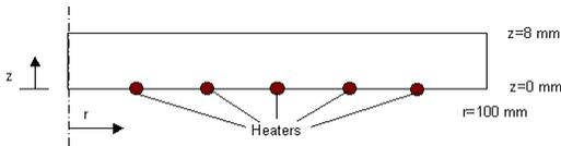
Figure 2. Schematic of axisymmetric, two-dimensional model of meter plate cross-section.
