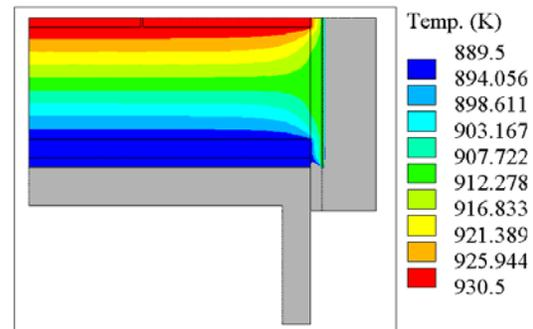
Figure 14. Temperature contours in 100 mm specimen for a temperature difference of 40 K at a mean temperature of 910 K.
