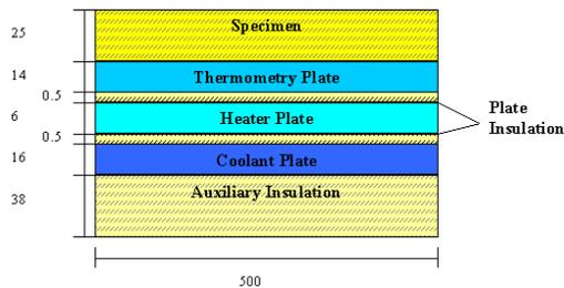
Figure 9. Schematic of composite cold plate (not to scale, dimensions in mm).
