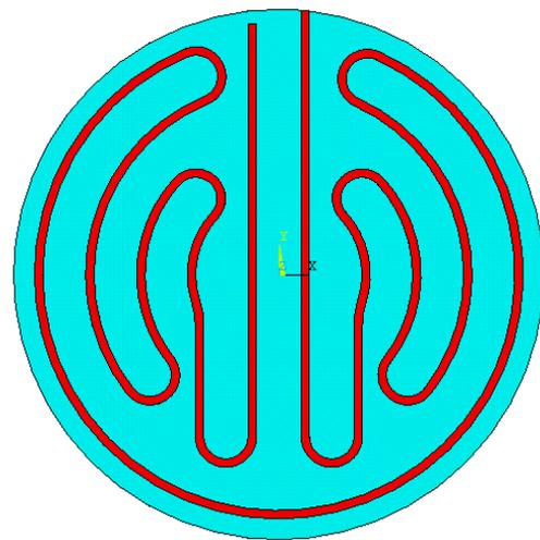
Figure 7. Final heater layout in meter plate.
