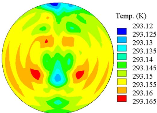
Figure 5. Temperature contours on surface of meter plate for original heater layout.
