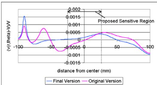
Figure 6. Temperature along path coincident with axis of SPRT for both heater layouts.
