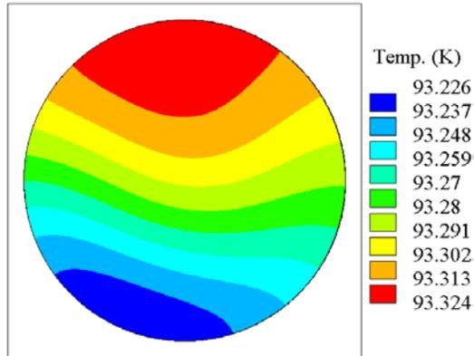
Figure 12. Temperature contours on surface of cold plate; nitrogen gas as coolant.
