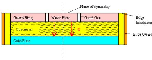
Figure 1. Simplified schematic of Guarded Hot Plate cross section.
