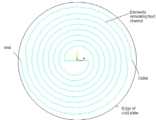
Figure 10. Fluid elements in cold plate
