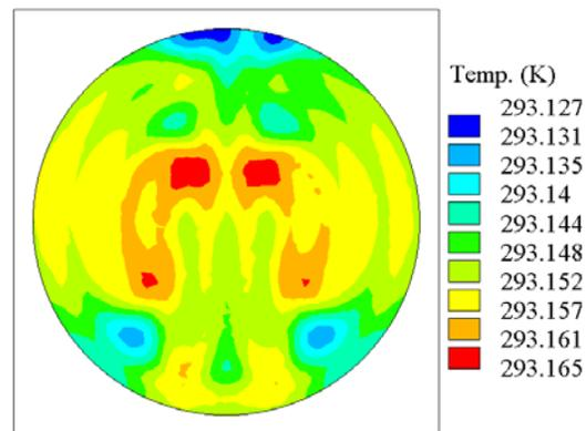
Figure 8. Temperature contours on surface of meter plate for final heater layout.
