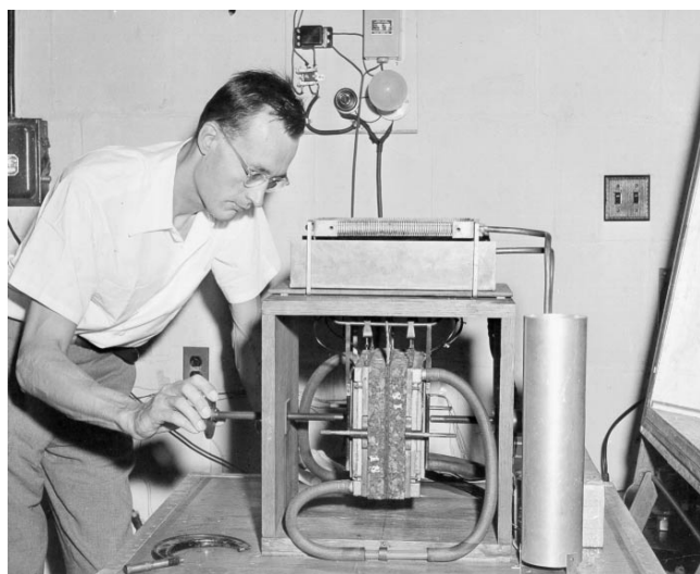
Figure 2 Henry E. Robinson (1911-1972) installs a pair of corkboard specimens for interlaboratory testing (c. 1948).
