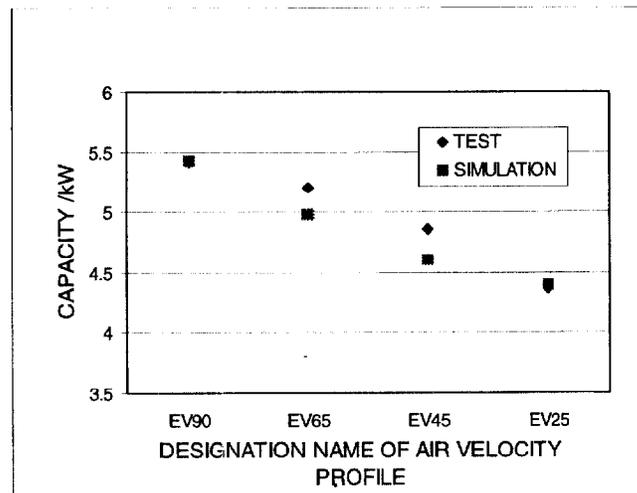
**Figure 1:** Model validation for different inlet air distributions
