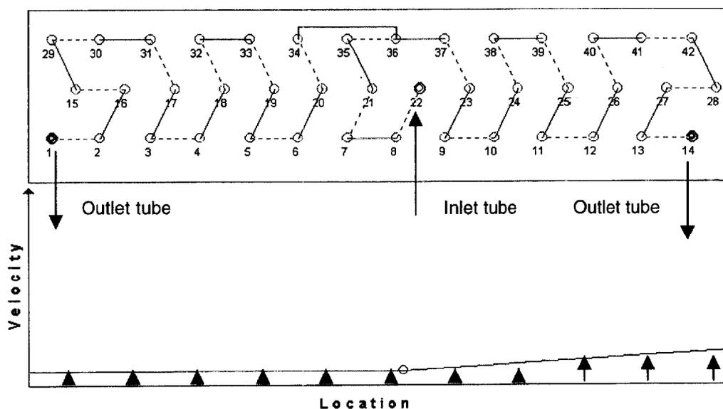
**Figure 2:** Side view of evaporator with circuitry specification and air velocity profile
