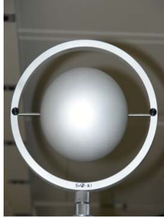
b. Spherical target - the spherical target is a 152 mm (6 in.) diameter spherically mounted retro-reflector (SMR). Front (left image) and back (right image) sides are shown.
