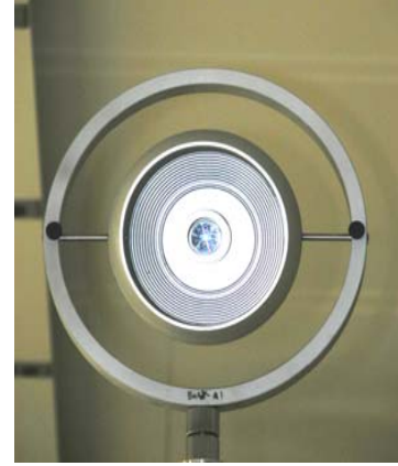
b. Spherical target - the spherical target is a 152 mm (6 in.) diameter spherically mounted retro-reflector (SMR). Front (left image) and back (right image) sides are shown.
