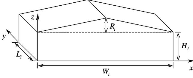
Figure 1. Schematic of gable-roofed building model with full-scale dimensions indicated.
