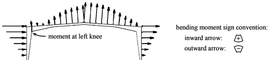
Figure 4. Influence coefficients associated with bending moment at left knee. Vectors show bending moments resulting from a unit force *inward* at each girt/purlin location.
