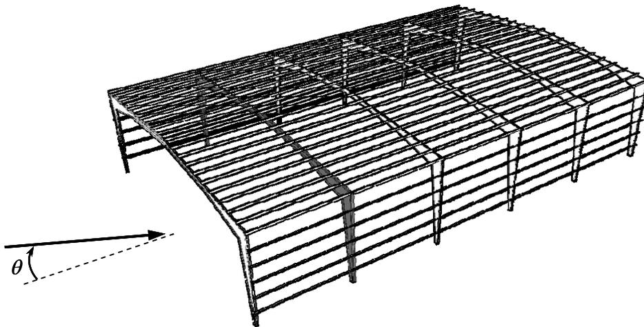
Figure 3. Perspective view of structural system showing frames, girts, and purlins (first interior frame highlighted).
