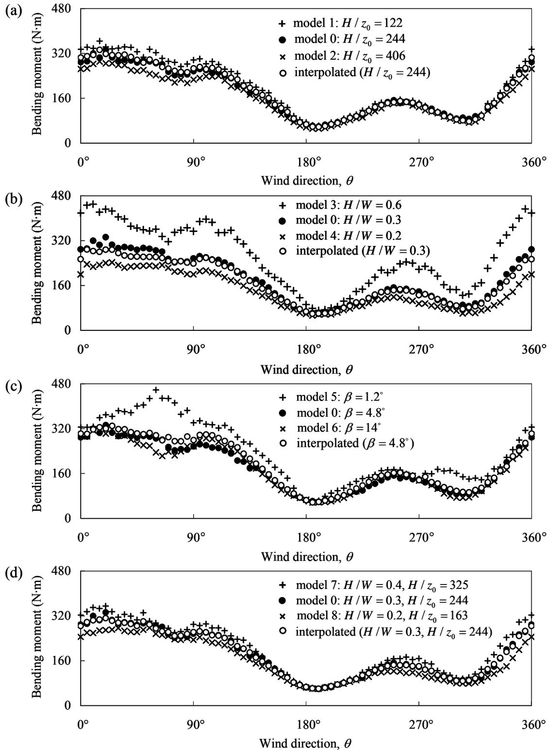
Figure 5. Maximum values of bending moment at the left knee of the first interior frame for the four interpolation test cases of Table 2: (a) case A; (b) case B; (c) case C; (d) case D. (Values correspond to an hourly averaged wind speed of 1 m/s at eave height.)
