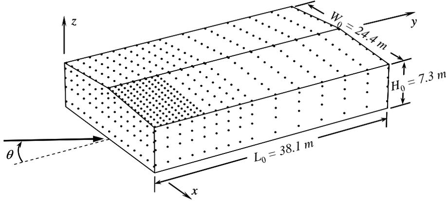
Figure 2. Perspective view of wind tunnel model showing tap locations, wind direction  $\theta$ , and full-scale building dimensions (1:12 roof slope).
