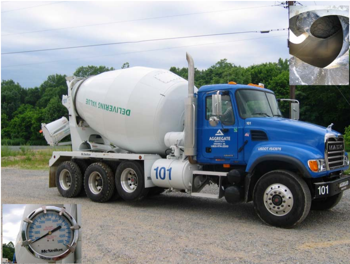
Figure 2: View of the truck used, the slump indicator, and the interior of the drum
