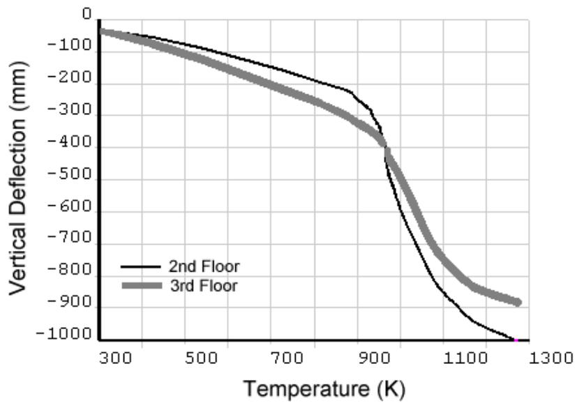
Fig. 3 Vertical deflections (mm) of second and third floors vs. temperature (°K)
