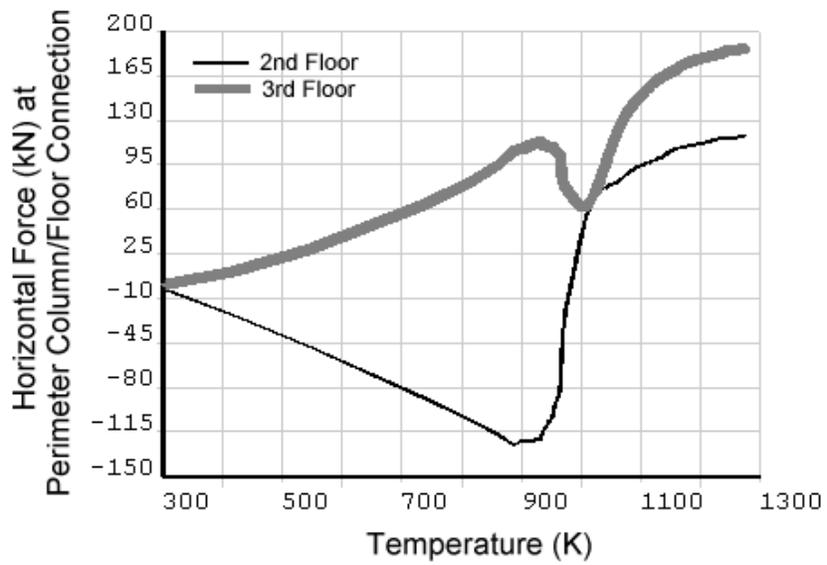
Fig. 2 Horizontal force (kN) between column and second and third floors vs. temperature (°K)
