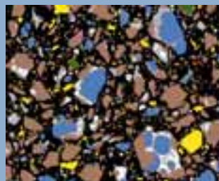
Figure 1. (a) Backscattered electron SEM image of a polished section of cement 140 from the Cement and Concrete Reference Laboratory proficiency sample program. (b) False color image of the same section, based on X-ray microprobe analysis. The meaning of each color is indicated in the accompanying legend. Images are 256 μm x 256 μm
