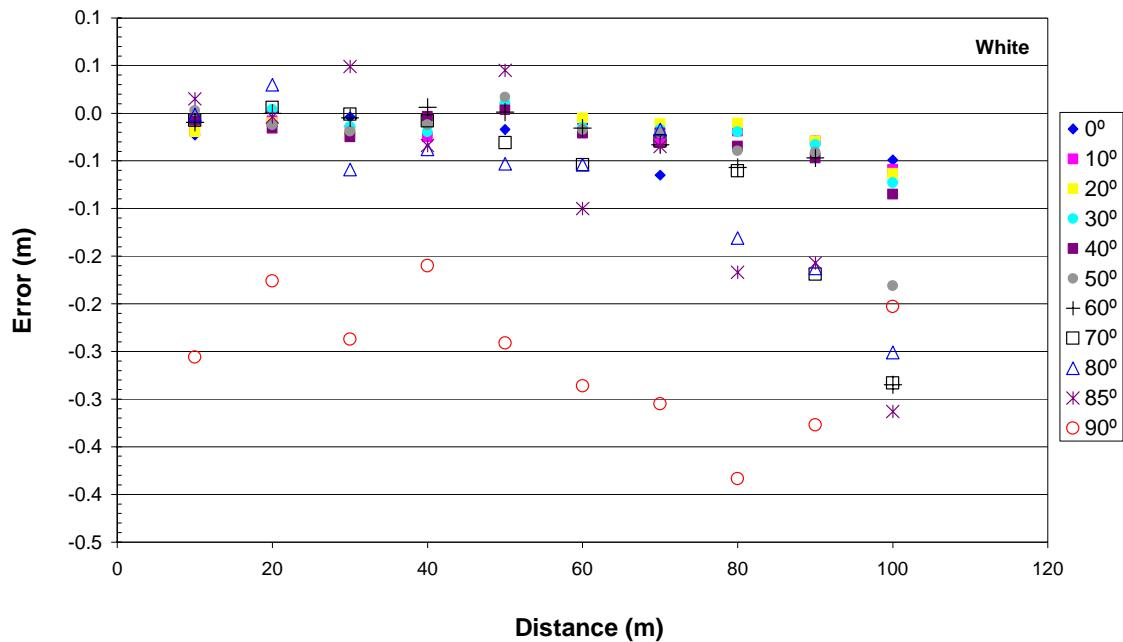
Figure 3.15a. Data Set 6: White Target – Error vs. Distance and Angle of Incidence.
