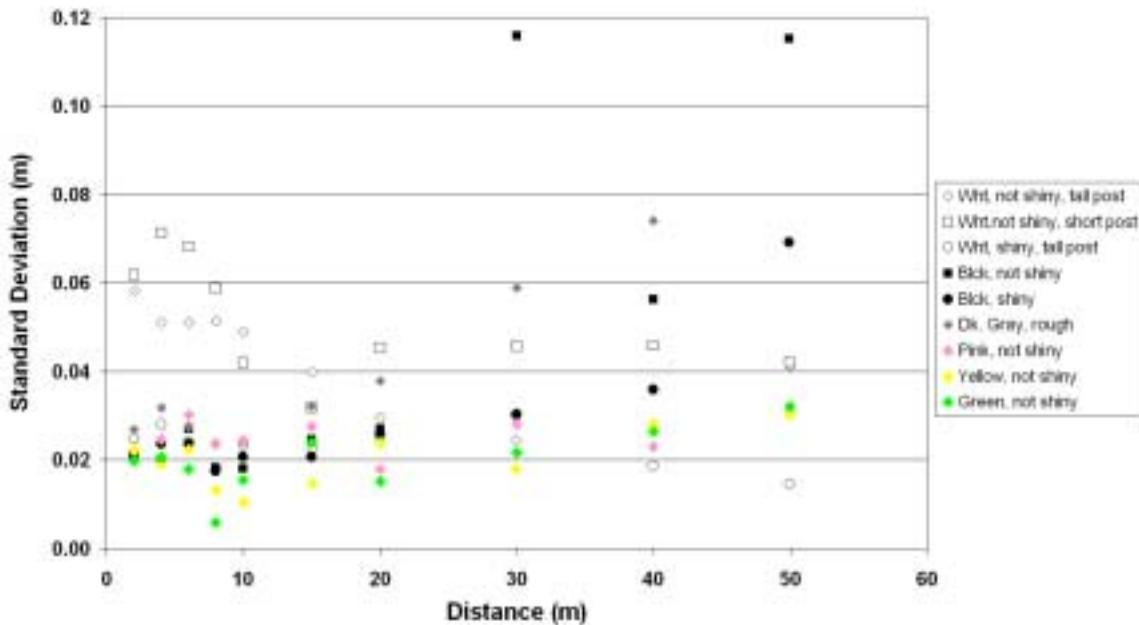
Figure 3.2. Data Set 1: Standard Deviation of Laser Measurements.
