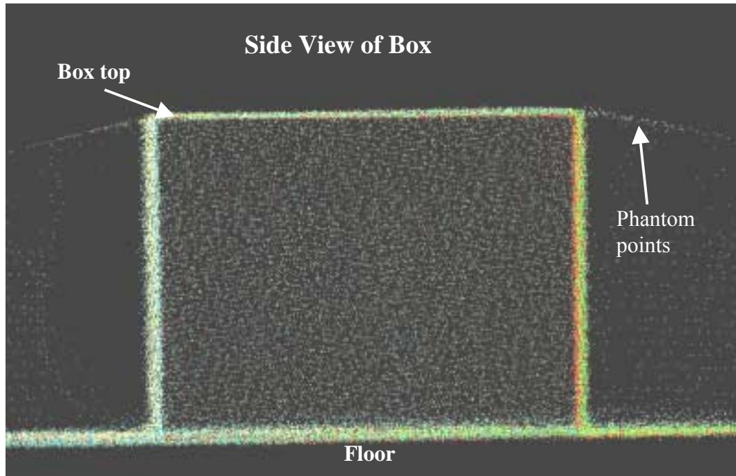
Figure 2.4. Point Cloud of Box Showing Phantom Points.
