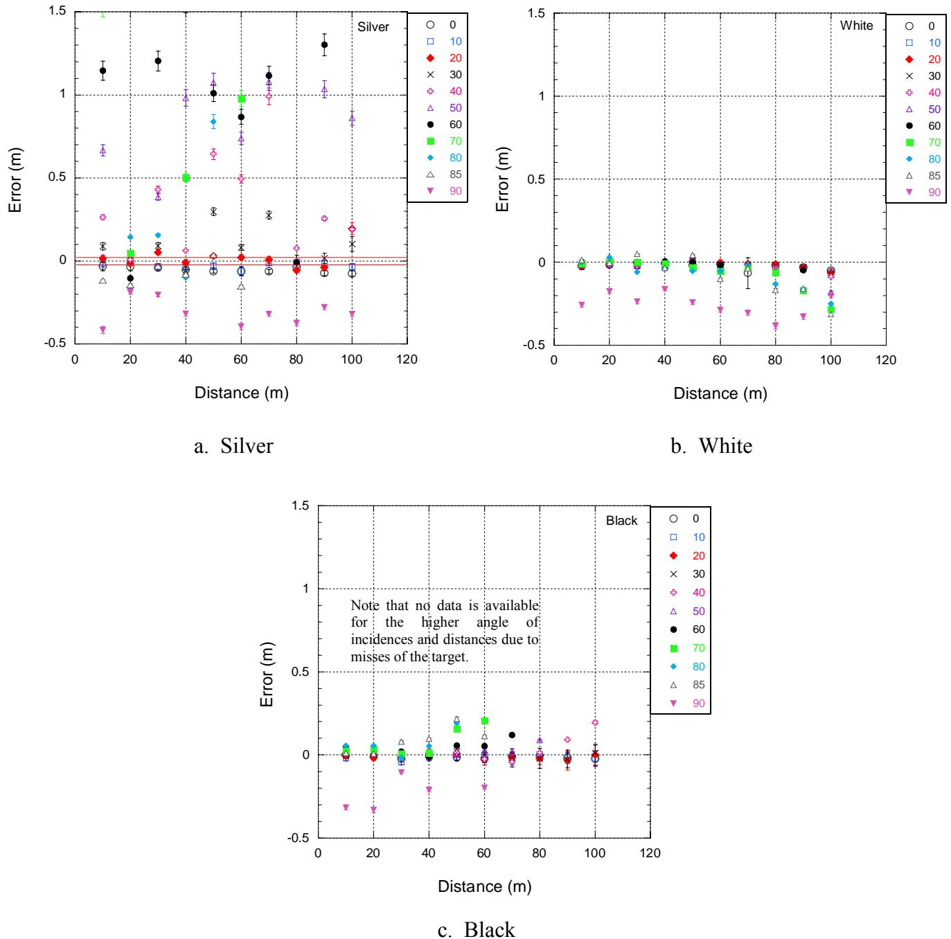
Figure 3.17. Data Set 6: Error vs. Distance and Angle of Incidence. Values in legend represent target rotation in degrees. (Error bars =  $1\sigma$ ).
