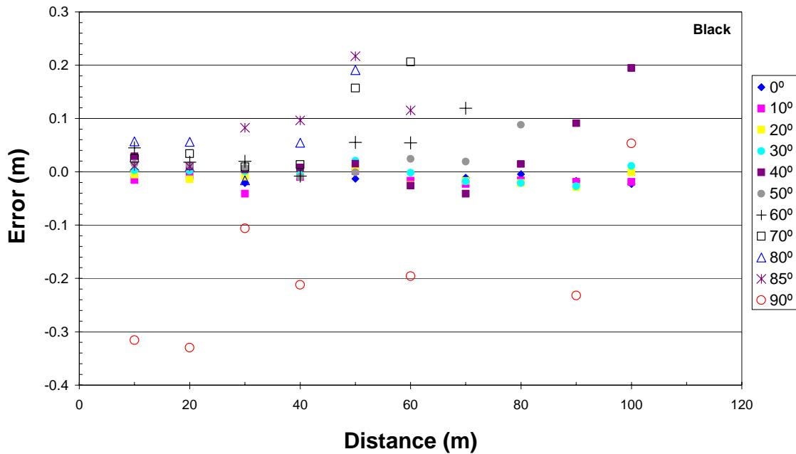
Figure 3.15b. Data Set 6: Black Target – Error vs. Distance and Angle of Incidence.
