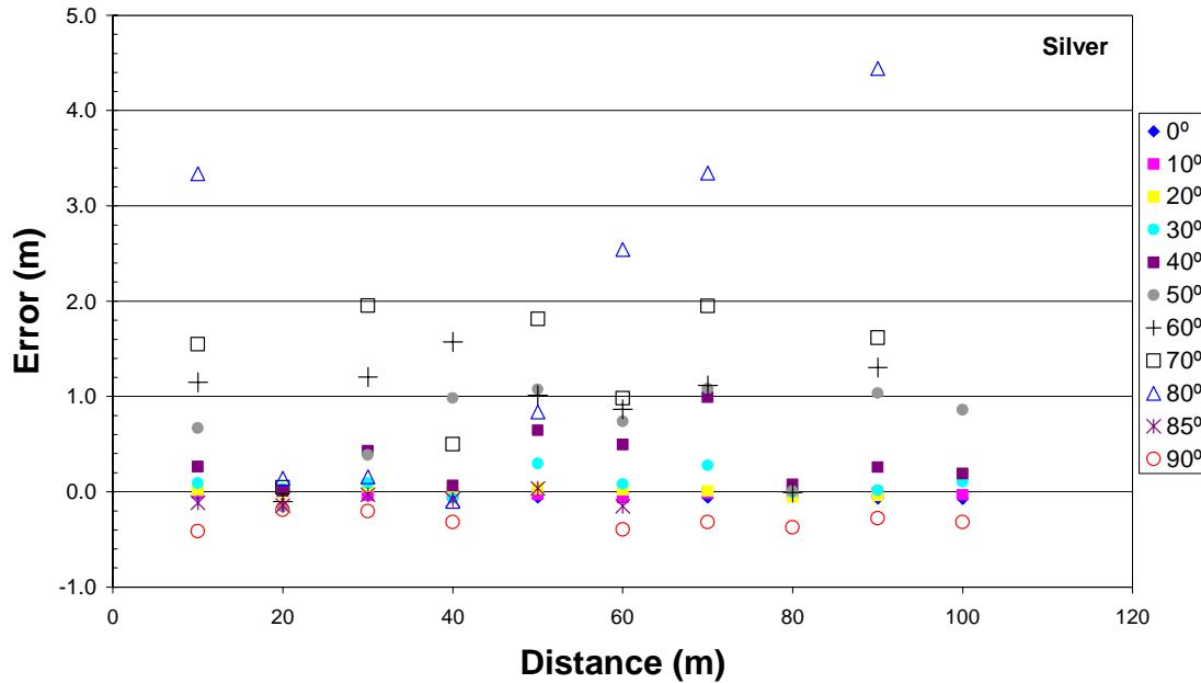
Figure 3.14a. Data Set 6: Silver Target – Error vs. Distance and Angle of Incidence.
