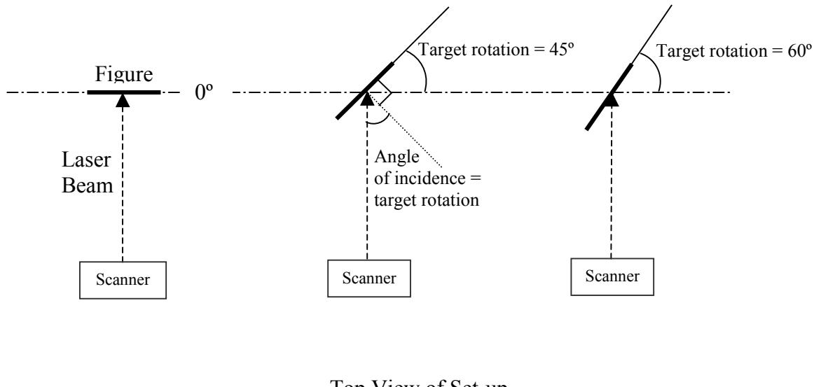
Figure 2.3. Rotation Orientation of LDP Target.
