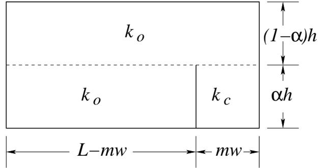
Figure 2: Crack model schematic for a concrete slab with span  $L$ , depth  $h$ , and containing  $m$  cracks, each of width  $w$ .  $k_o$  is the permeability of the uncracked concrete, and  $k_c$  is the permeability of each crack.
