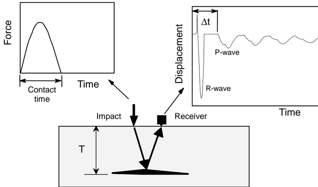
**Fig. 3— The impact-echo method: mechanical impact is used to generate stress waves and a receiver next to the impact point measures the resulting surface motion.**
