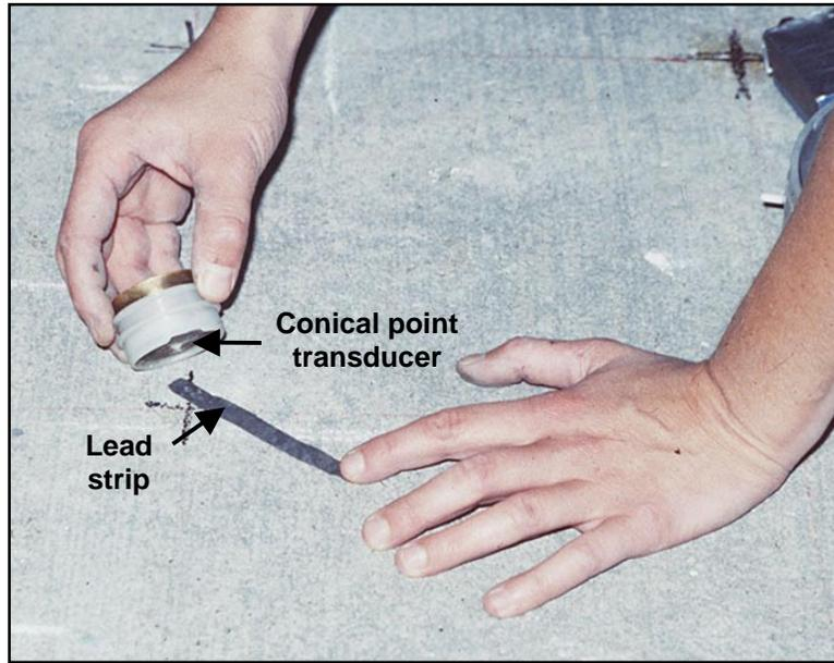
**Fig. 7— The NBS conical point displacement transducer being coupled to a concrete surface using a thin lead strip.**
