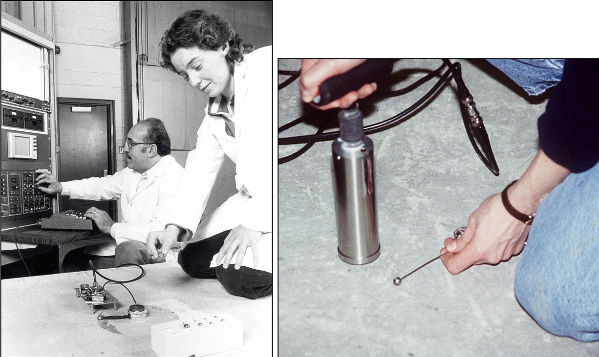
**Fig. 6— (Left) In the early research steel balls were used to obtain impacts with different contact times; (Right) steel balls mounted on spring-steel rods are suited for field-testing.**
