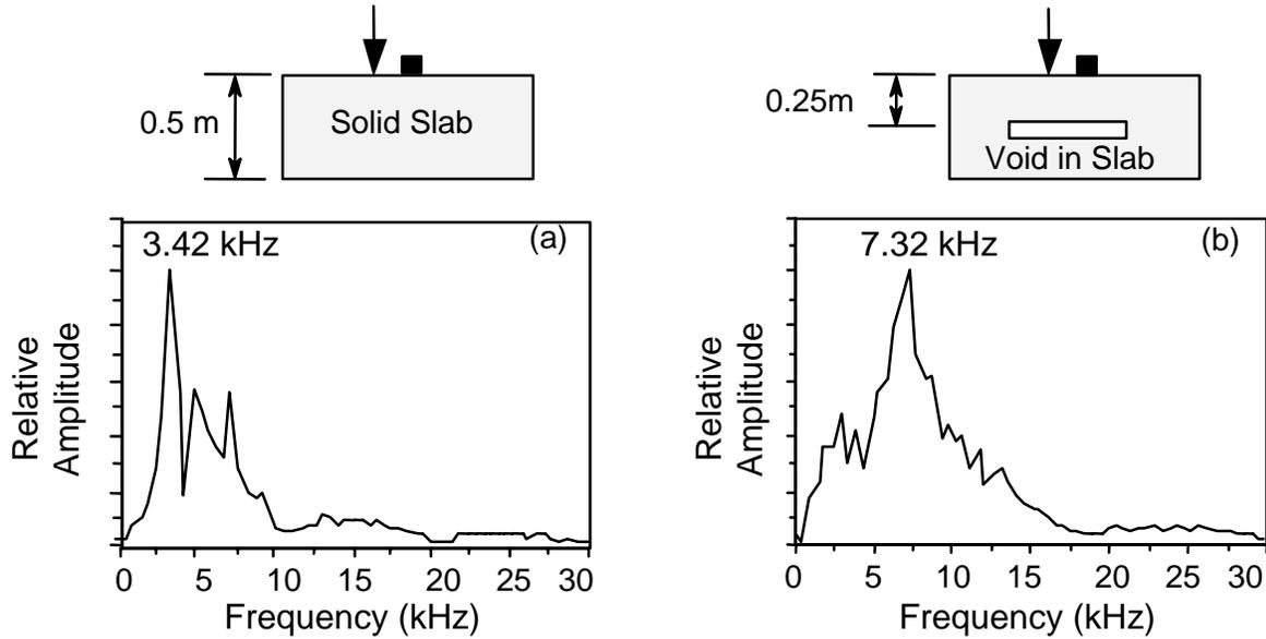
**Fig. 5— Examples of amplitude spectra from impact-echo tests: a) test of solid portion of a 0.5 m thick slab and b) test over an artificial void approximately 0.25 m deep.**
