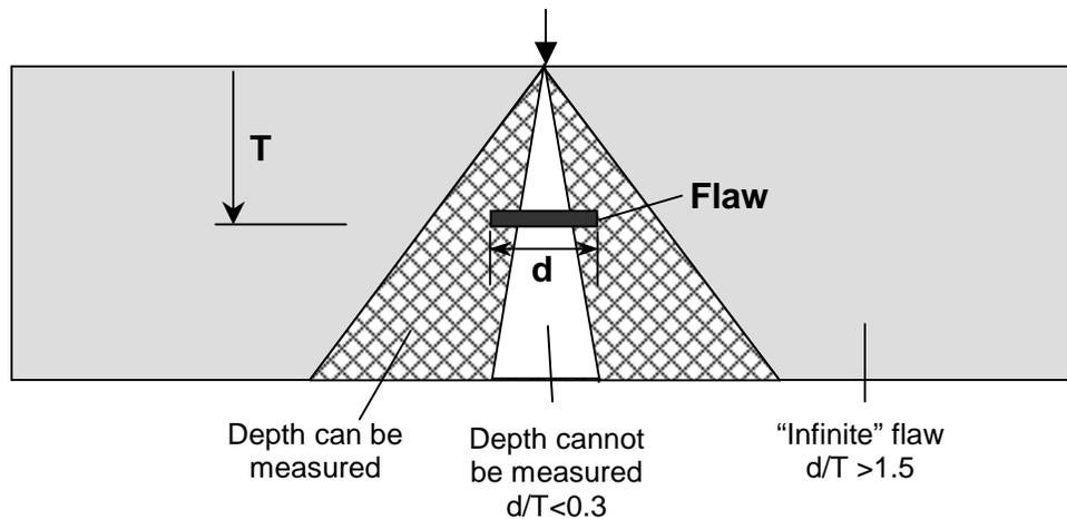
**Fig. 10—The smallest detectable horizontal crack or void depends on its depth; if the flaw falls within the white region, its depth cannot be measured (based on Sansalone and Streett [1997]).**
