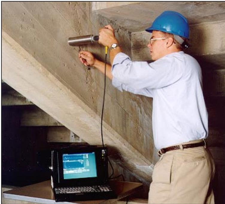
**Fig. 8— Example of PC-based impact-echo test equipment (courtesy of Impact-Echo Instruments, LLC).**
