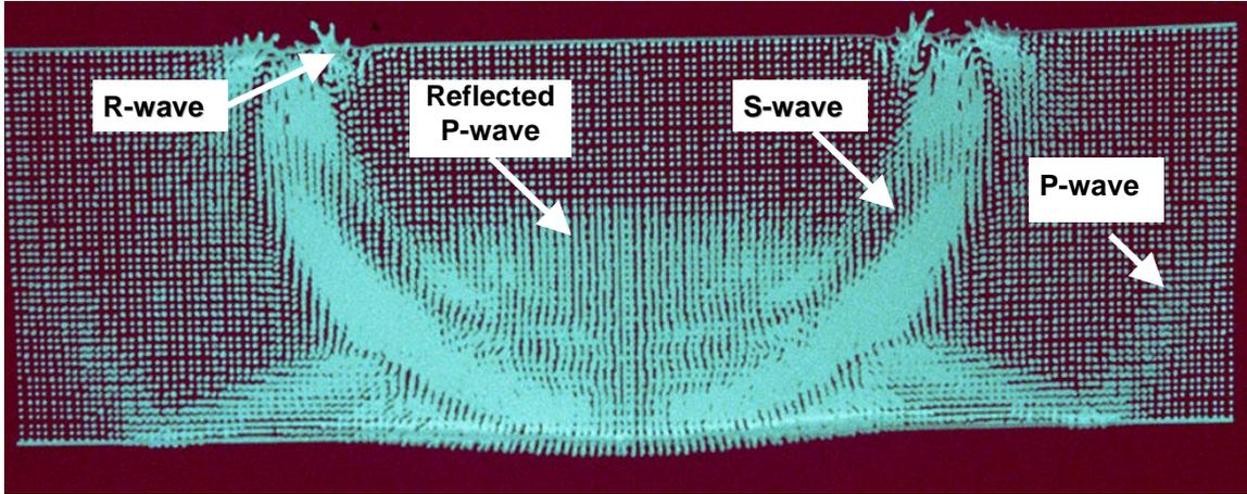
**Fig. 2—Finite element simulation of impact on a plate; at this point in the analysis the S-wave front is arriving at the bottom of the plate and the P-wave has reflected halfway up the plate.**
