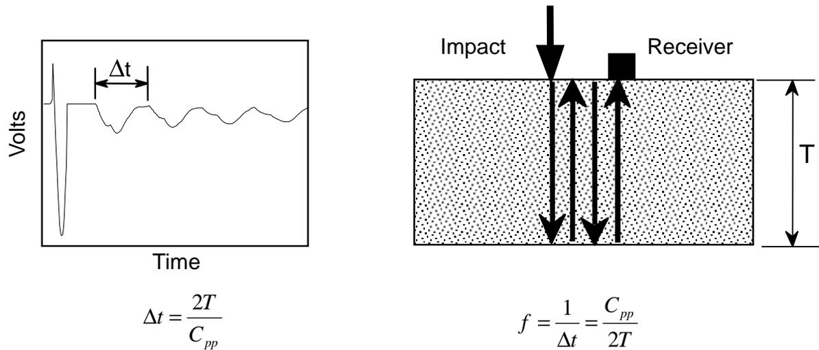
**Fig. 4— Principle of frequency analysis: the time domain waveform has a periodic pattern due to P-wave arrival as it undergoes multiple reflections between the top and bottom of the plate; the frequency of P-wave arrival is related directly to the plate thickness.**
