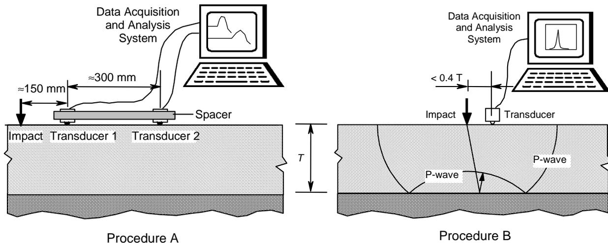
**Fig. 11—Two-step procedure for measuring plate thickness according to ACTM C 1383: Procedure A is used to determine the P-wave speed and Procedure B is used to determine the thickness frequency.**
