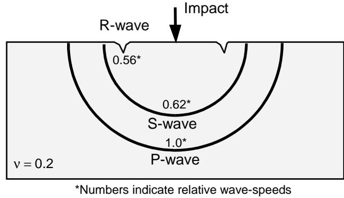
**Fig. 1—Stress waves caused by impact at a point on the surface of a concrete plate.**
