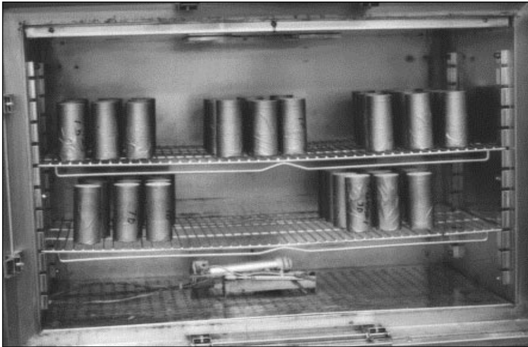
Figure 5—Specimens covered with plastic tape stored in environmental chamber
