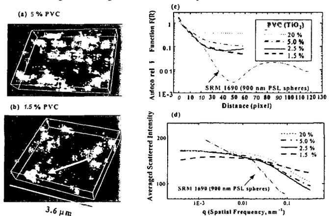
**Figure 2.** (a)-(b) 3D reconstruction images for the 5% and 2.5% PVC TiO<sub>2</sub> pigmented samples. (c) Autocorrelation function F(R), and (d) circularly averaged scattered intensity obtained from Fast Fourier transformation (FFT) of LSCM images in Fig.1 for four different PVC samples.
