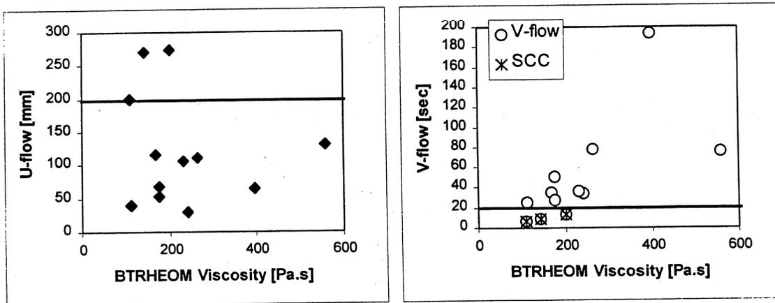
**Figure 3: U-flow and V-flow time compared with viscosity measured with the BTRHEOM.**
