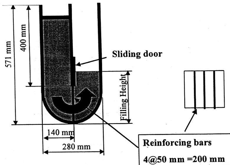
*Figure 1. U-flow test*
