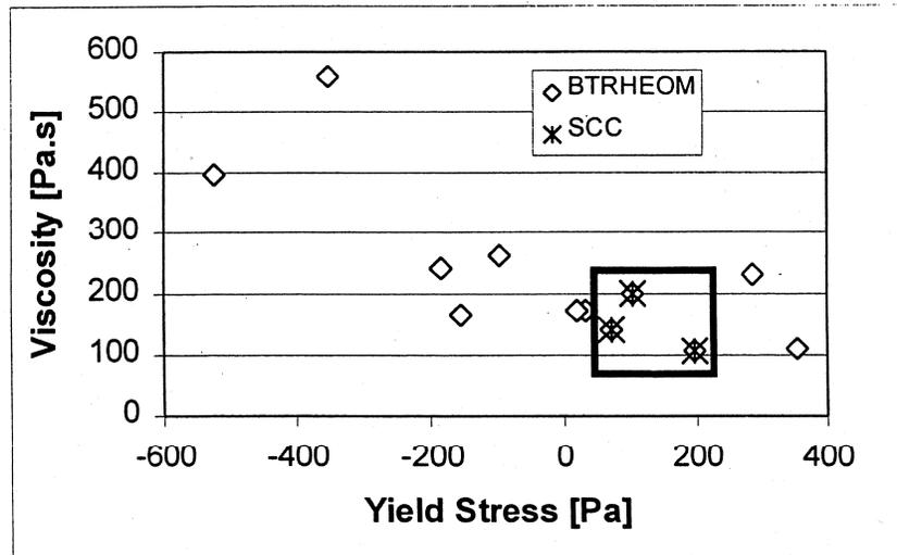
*Figure 4: Viscosity vs. Yield stress calculated according to Bingham equation and the workability box*
