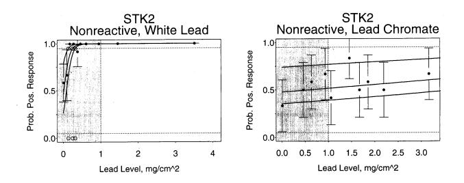
Figure 2. Probability of a Positive Response Versus Lead Level for Spot Test Kit 2 (STK2) for Each Operator. (The filled circles represent the proportions of positive responses at a given lead level, and the error bars are the associated 95 % binomial confidence intervals. The two horizontal dashed lines represent the 0.5 and 0.95 probabilities of a positive response. Circles are the 0.95 probability point for each operator; they are repeated above the horizontal axis for clarity.)
