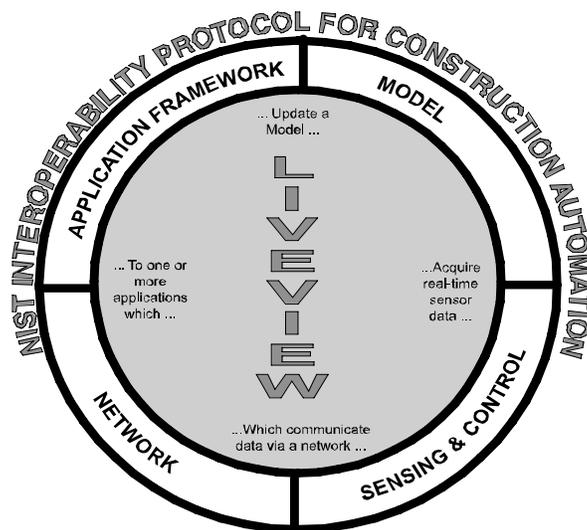
Figure 1: LiveView is comprised of 4 interconnected areas which will permit plug-and-play remote sensing at the construction site.
