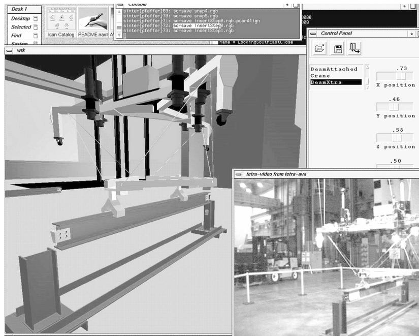
Figure 2: Augmented Simulation mirror-world at the National Construction Automation Testbed, located on the NIST campus in Gaithersburg, Maryland. Live scenes from an 8-DOF robotic crane are shown at lower right via closed circuit video. A real-time data stream, uplinked using the LiveView interoperability protocol, is used to drive the motion of the Virtual Site Simulator at left which provides live 3D viewing of construction site activity.
