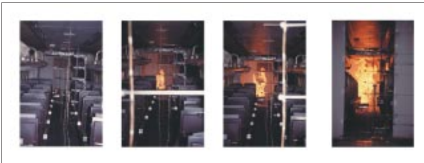
Fire growth in real-scale gas burner fire tests in a passenger rail coach car.
