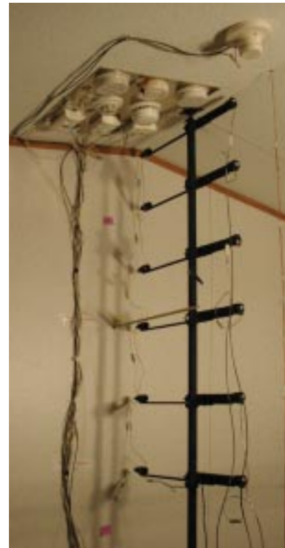
Instrumentation for smoke alarm tests in a manufactured home.
