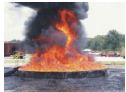
Test burn to study effects of intentional burning of oil spills in marshland environment.
