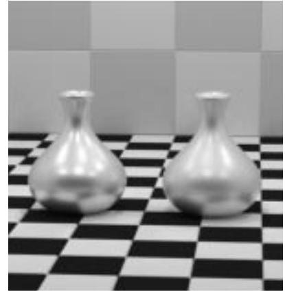
Vases rendered with two different metallic-flake pigmented coatings. The vase on the left is coated with a material having larger flakes than the one on the right and appears more specular, consistent with reflectance measurements.
