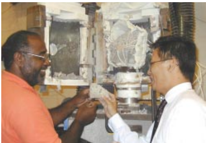
Mr. Frank Davis and Dr. Long Phan examine a concrete specimen tested at high temperature.
