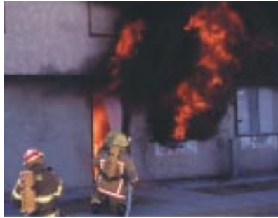
Burn of instrumented townhouse for arson investigation study.
