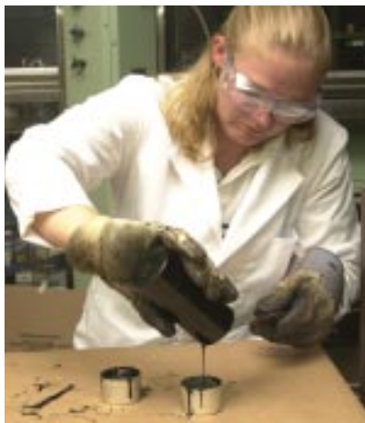
AMRL research associate Kathryn Tice preparing hot performance graded asphalt binder test samples for placement in a pressurized aging vessel.
