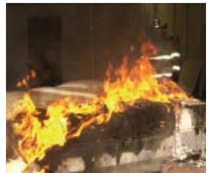
Bed fire about two minutes after ignition with a match sized flame.
