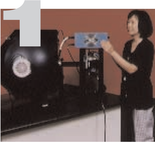
Advanced photodegradation device capable of exposing polymeric materials to a highly, spatially uniform ultraviolet radiant flux.
