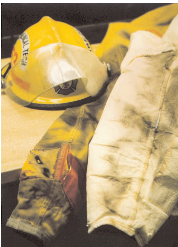
Fire Fighter turnout gear damaged during a fire that resulted in burn injuries
