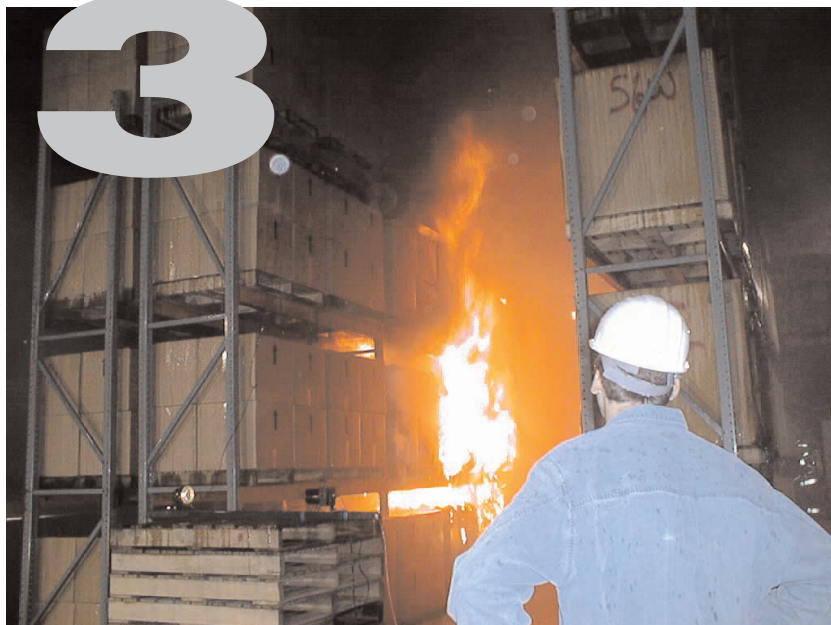
Fire Test of interaction of sprinklers, draft curtains and heat and smoke vents
