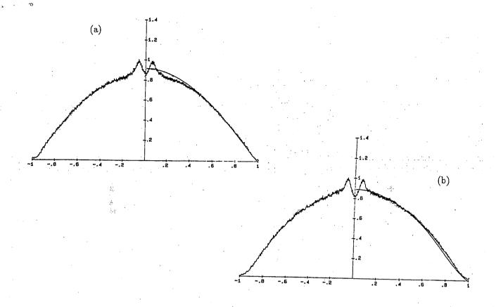
Figure 1: (a) Measured (noisy) and theoretical (smooth) input near-field distribution for overfilled launch. (b) Output near-field distributions measured (noisy) and calculated from the transfer function (smooth).
