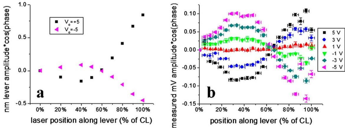
Fig. 3. Simulated (a) and experimental results (b) of the measured first harmonic response of a cantilever to periodic tip/lever biasing as a function of position along the lever and DC offset.
