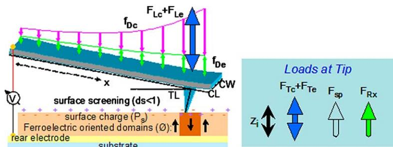
Fig. 1. Sketch of long range distributed loads, surface actuation, and tip loads acting on an integrated tip and cantilever during PFM.
