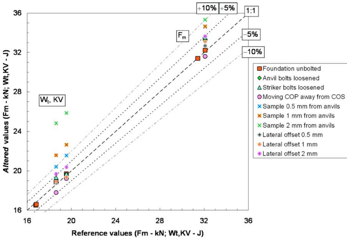
FIG. 2—Effect of test machine variables and specimen positioning for brittle specimens (low-energy level at RT and  $-40^{\circ}\text{C}$ ).
