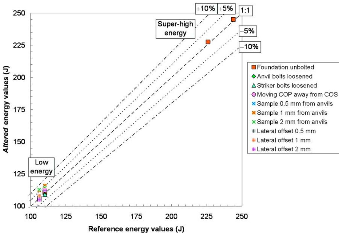
FIG. 4—Effect of test machine variables and specimen positioning on absorbed energies for ductile specimens (high- and super-high energy).
