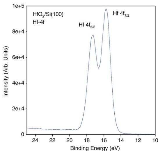
Fig. 1. Hf-4f XPS spectra for the PLD synthesized  $\text{HfO}_2/\text{Si}(100)$  films. The 4f spin-orbit splitting and intensity ratio of  $4f_{7/2}$  and  $4f_{5/2}$  are in agreement with theoretical expectations.
