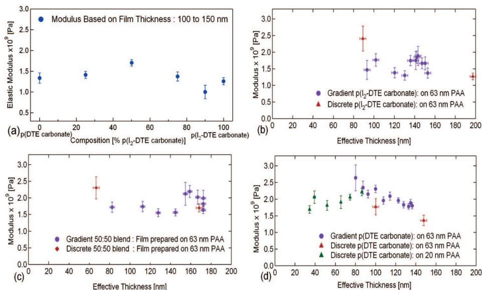
**Figure 5.** Elastic moduli of the respective polymer films. (a) Modulus as a function of composition for films 100–150 nm in thickness. (b–d) Modulus of p(I<sub>2</sub>-DTE carbonate), 50:50 blend and p(DTE carbonate) films as a function of thickness based on post-transfer film thicknesses to PDMS. Modulus error bars is  $\pm 1$  unit standard deviation. Thickness error is  $\pm 2$  nm.
