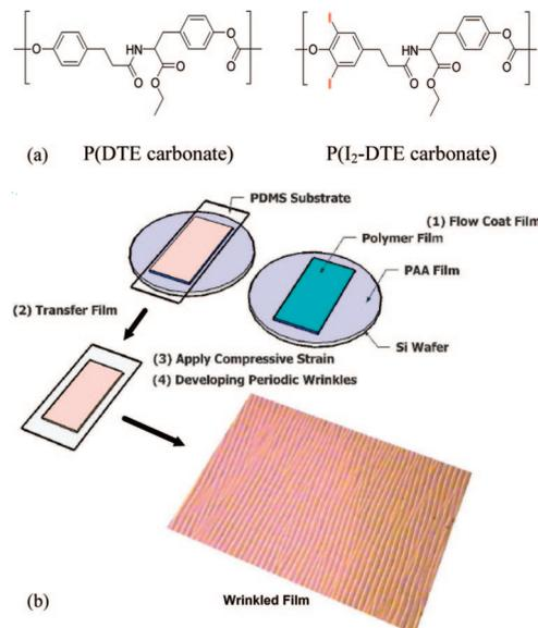
**Figure 2.** (a) Scheme showing chemical structures of p(DTE carbonate) and p(I<sub>2</sub>-DTE carbonate) polymers. (b) Schematic presentation of the steps involved in the SIEBIMM technique.
