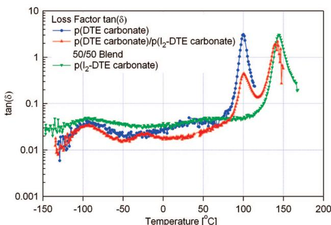
**Figure 1.** Temperature dependence of the loss tangent ( $\tan(\delta)$ ) in dynamic stress relaxation of p(DTE carbonate), p(I<sub>2</sub>-DTE carbonate), and their 50:50 mass % blend in the tension mode at a frequency of 1 Hz. Shown are the  $\alpha$ -( $T_g$ ) and the  $\beta$ -relaxation behavior of both polymers.
