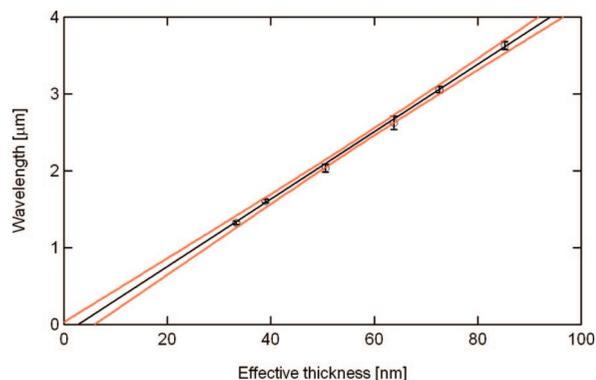
**Figure 6.** Wavelength of the wrinkles as a function of film thickness from the p(DTE carbonate) discrete film thickness series. Solid line represents best fit of data (black) and the 95% confidence bands (red).
