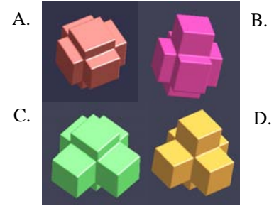
Figure 2: Four types of unit cells found in CWRU and Mayo scaffold. A) No long axis, B) 1 long axis, C) 2 long axes, D) 3 long axes.
