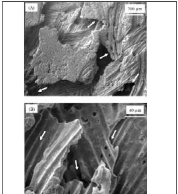
**Figure 2.** SEM of pore channels in CPC-suture fiber composite scaffold after suture fiber dissolution. Arrows indicate the flow of the interconnected pore channels beneath the CPC surface.
