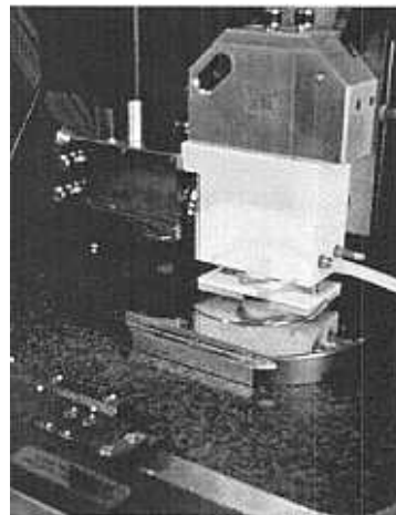
Figure 1. Environment chamber attached to a scanning stylus AFM
