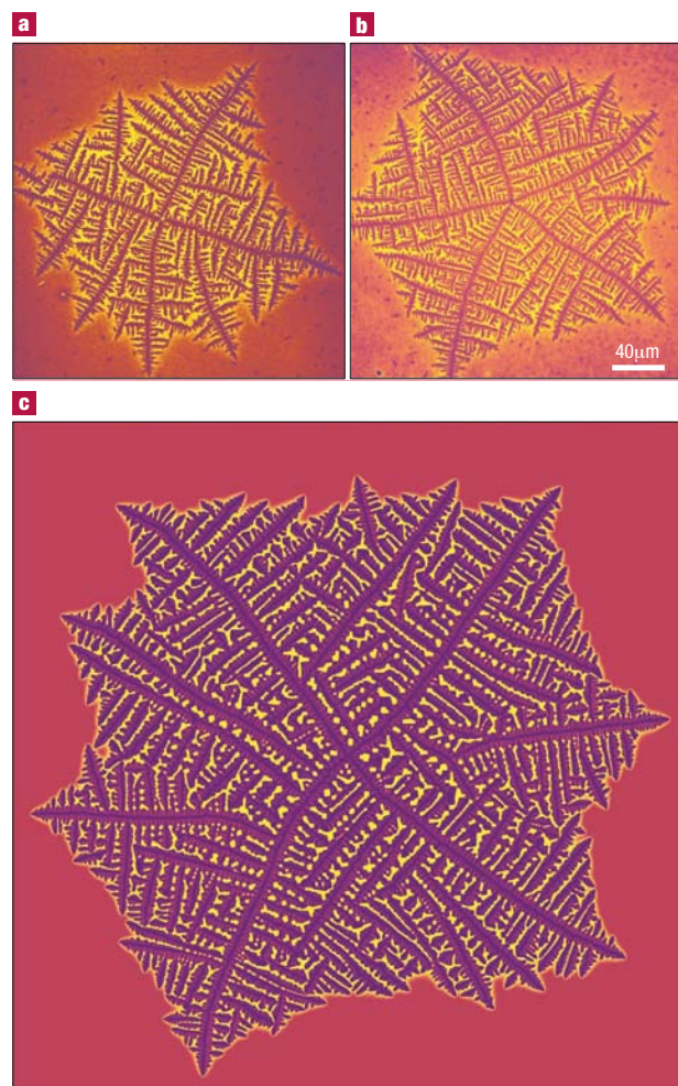
Figure 2 'Dizzy' dendrites. a,b , Growth shapes formed in 80-nm-thick films of a clay-PEO/PMMA blend with 15% relative mass of clay to polymer. c , Composition map from a phase-field simulation on a 3,000 \times 3,000 grid ( 39.4 \mu\text{m} \times 39.4 \mu\text{m} ) using 18,000 single-pixel orientation-pinning centres distributed randomly. (The same scale applies for a and b .)
