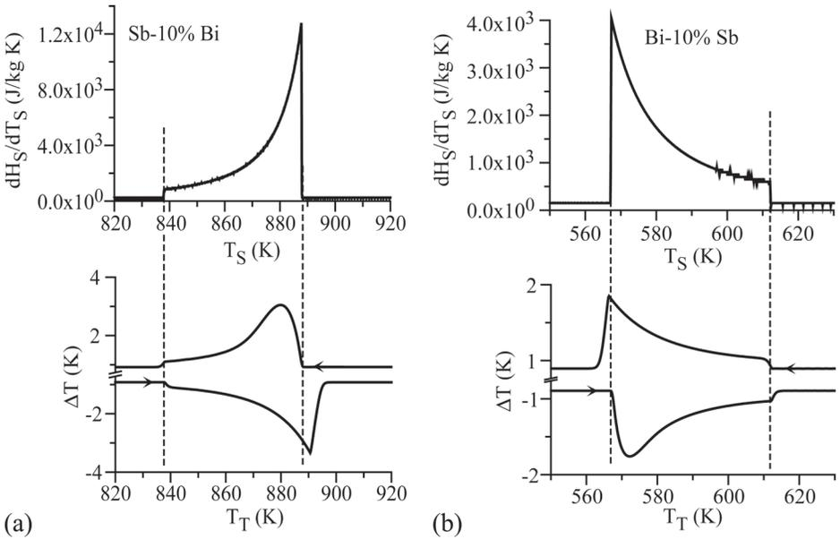
**Figure 3.14.** Comparison of Bi-10% Sb with  $k > 1$  and Sb-10% Bi with  $k < 1$  alloys. The  $dH_S/dT_S$  curves computed for lever law using the thermodynamic functions of [92Feu] and the computed DTA scans for heating and cooling are shown.
