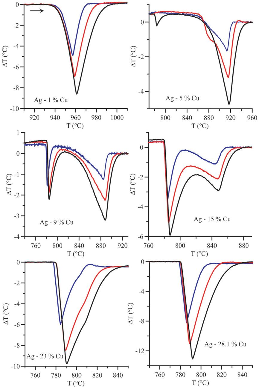
**Figure 3.3.** Experimental DTA melting scans for a series of Ag-Cu alloys at three different heating rates, 5 K/min (blue), 10 K/min (red) and 15 K/min (black). Note that the small signal for the eutectic melting is absent in the Ag-5 % Cu alloy at the slower heating rates. Note also the absence of a distinct second peak in Ag-23 % Cu. Percentage is by mass.
