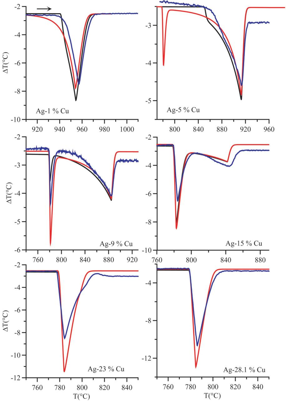
**Figure 3.4.** Computed DTA curves for Lever (black) and Scheil (red) at 5 K/min. The experimental DTA curves are shown blue. Lever and Scheil curves for two alloys are essentially identical and only the Scheil curve is shown for Ag-23 % Cu, and 28.1 % Cu.
