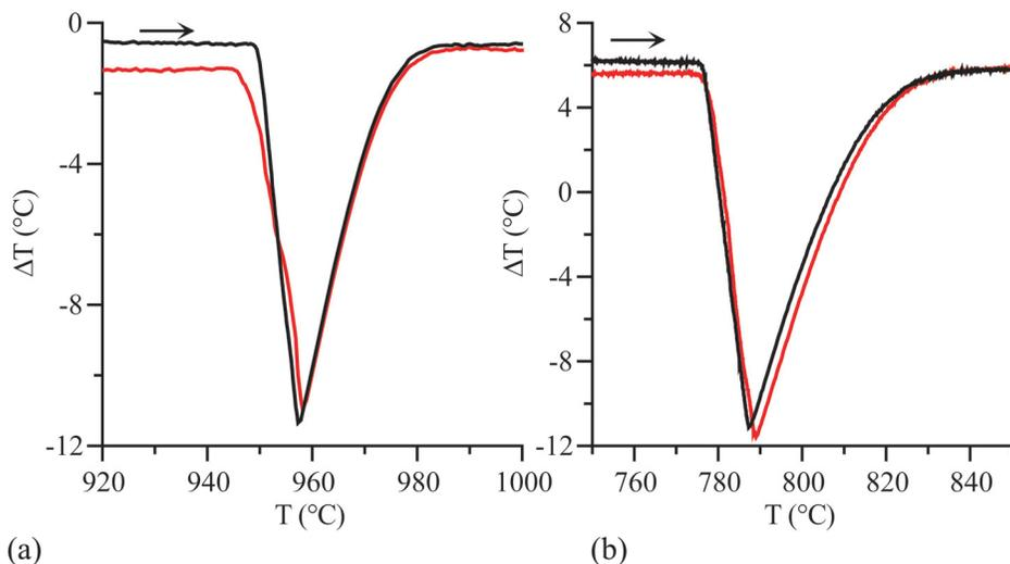
**Figure 2.4.** DTA signal for melting of (a) pure Ag (211.6 mg; 10 K/min) and (b) Ag-Cu eutectic (231.3 mg; 15 K/min) comparing first melt (red) and second melt (blue). Note the offset of the baselines, the more rounded onsets and the lack of linearity of the down-slopes for the first melt compared to the second.
