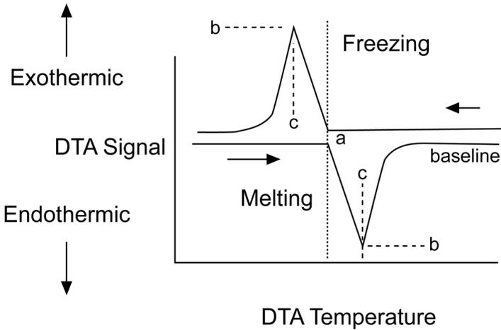
**Figure. 1.1** DTA responses to melting and freezing of a pure material under ideal conditions. *a*-onset temperatures (taken here as equal to the melting point,  $T_M$ ), *b*-peak signals, *c*-peak temperatures.
