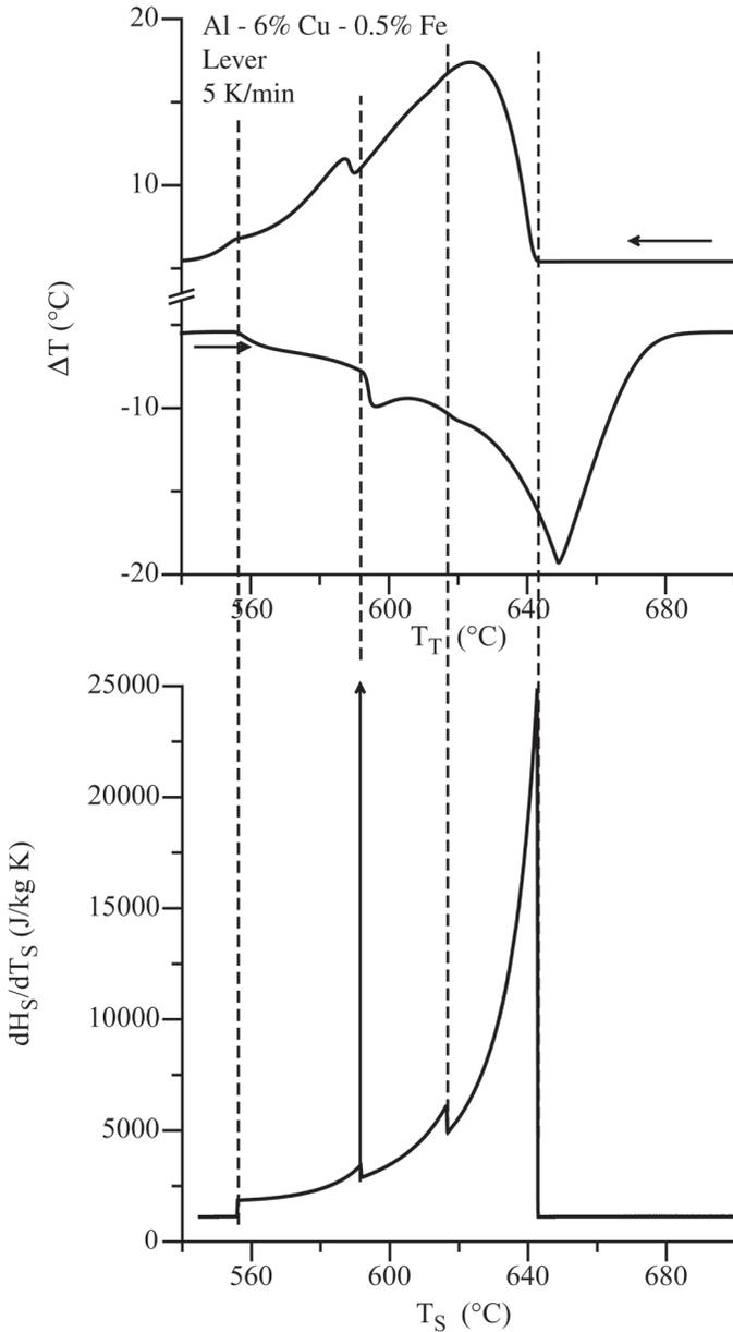
**Figure 4.3.** DTA and  $dH_S/dT_S$  plots for Al-6 % Cu-0.5 % Fe under equilibrium conditions. The aluminum alloy thermodynamic database [96Sau1] was employed. The solidification sequence is:  $L \rightarrow FCC$ ,  $L \rightarrow FCC + Al_6(Fe, Cu)$ ,  $L + Al_6(Fe, Cu) \rightarrow FCC + Al_7Cu_2Fe$ ,  $L \rightarrow FCC + Al_7Cu_2Fe$ . Note the delta function at  $\approx 592^\circ C$  corresponding to the invariant reaction,  $L + Al_6(Fe, Cu) \rightarrow FCC + Al_7Cu_2Fe$ .
