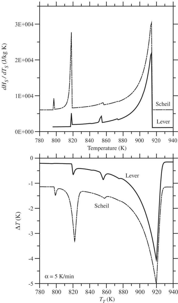
**Figure G2.** Top)  $dH_S/dT_S$  obtained from the enthalpy-temperature predictions for Al 2219 alloy computed using thermodynamic database [96Sau1] for lever and Scheil conditions for Al 2219 alloy. The curve for 'Scheil' is shifted by  $5 \times 10^3$  J/kg K for clarity. Bottom) Corresponding DTA plots for melting at 5 K/min. The curve for 'Lever' is shifted up 1 K for clarity.
