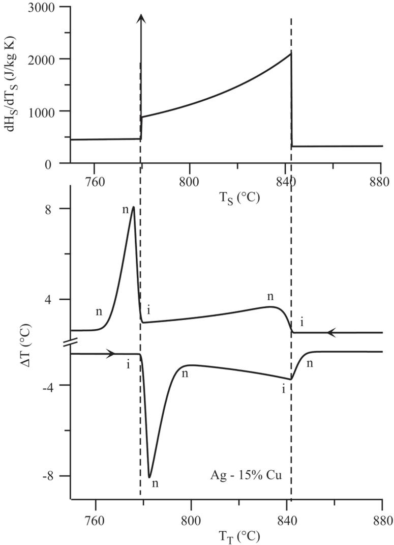
**Figure 3.9.**  $dH_S/dT_S$  vs.  $T_S$  (top) and computed DTA scans for melting and freezing at 5 K/min (bottom) for Ag- 15 % Cu using equilibrium enthalpy. Features on the DTA scans are labeled with: **i** = important or **n** = not important.
