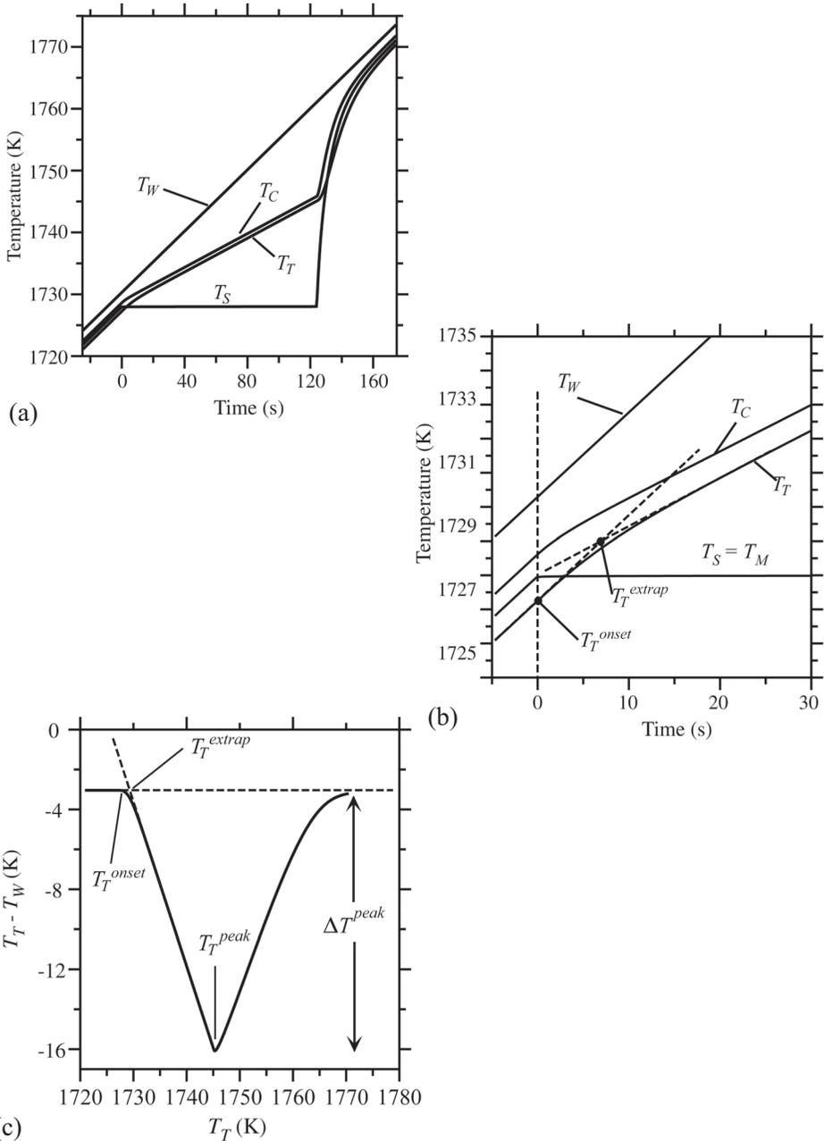
**Figure D1.** a) Calculated temperatures within a DTA instrument as functions of time for pure Ni, sample ( $T_S$ ), sample cup ( $T_C$ ), thermocouple ( $T_T$ ) and furnace wall ( $T_W$ ), b) enlarged region near  $t = 0$ , c) associated DTA curve. The figures show the possible sources of error in determining the melting onset temperature for calibration purposes.
