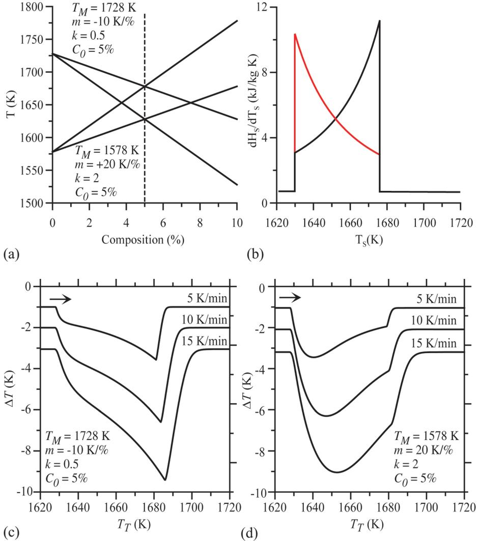
**Figure 3.13.** Comparison of two hypothetical alloys with identical heat of fusion, liquidus and solidus temperatures but differing having  $k < 1$  and  $k > 1$ . a) Phase diagram, b)  $dH_S/dT_S$  for  $k < 1$  (black) and  $k > 1$  (red), c) DTA for  $k < 1$  and d) DTA for  $k > 1$ . For  $k < 1$ , the latent heat is released higher in the freezing range compared to  $k > 1$  where the latent heat is related lower in the freezing range.
