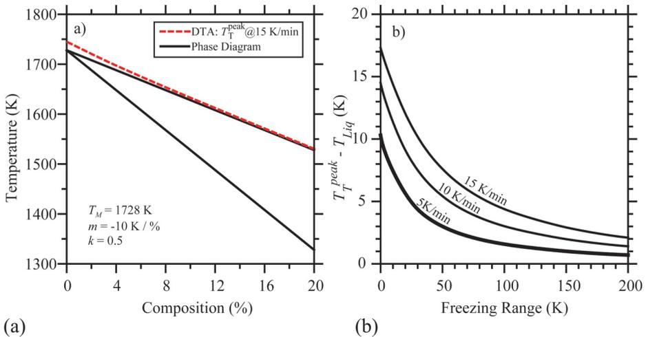
**Figure 3.11.** a) DTA peak temperature calculated at a heating rate of 15 K/min for different alloy compositions using a lever assumption. Peak temperature is superimposed on the phase diagram ( $T_M = 1728 \text{ K}$ ,  $m = -10 \text{ K} / \%$ ,  $k = 0.5$ ). b) The difference between the peak temperature and the liquidus temperature as a function of freezing range at three heating rates. The freezing range is given by  $mC_0 [(k - 1)/k]$ .
