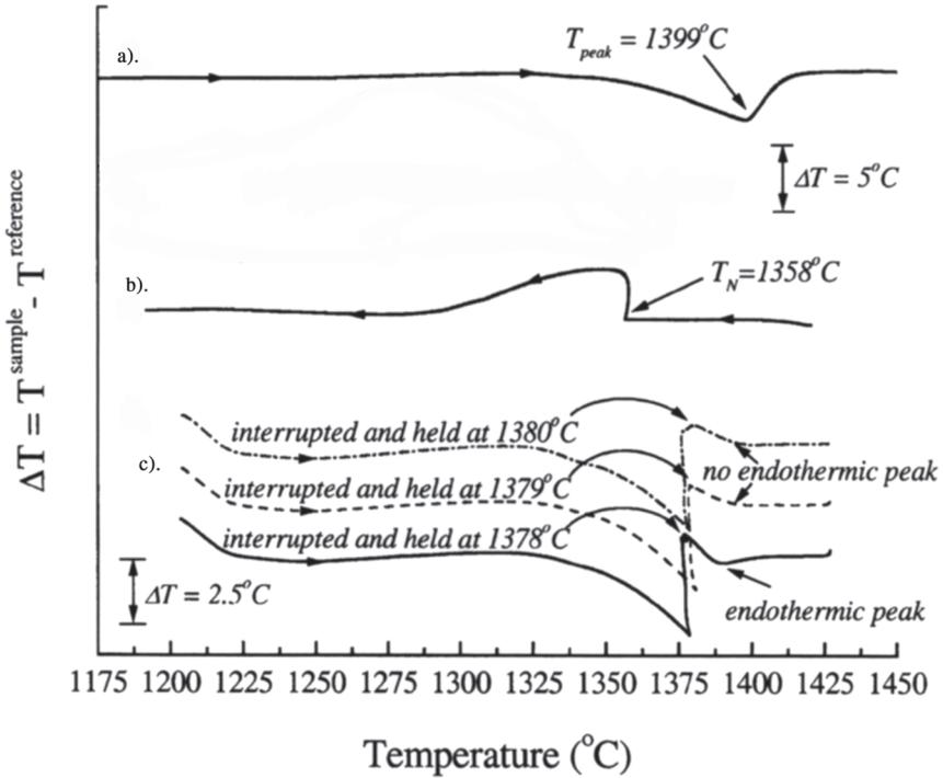
**Figure 3.12.** a) Normal DTA scan on heating for a small freezing range Ni-base superalloy; b) Normal DTA scan on cooling. Supercooling has occurred; c) Cycling DTA to determine the liquidus temperature [00Wu].
