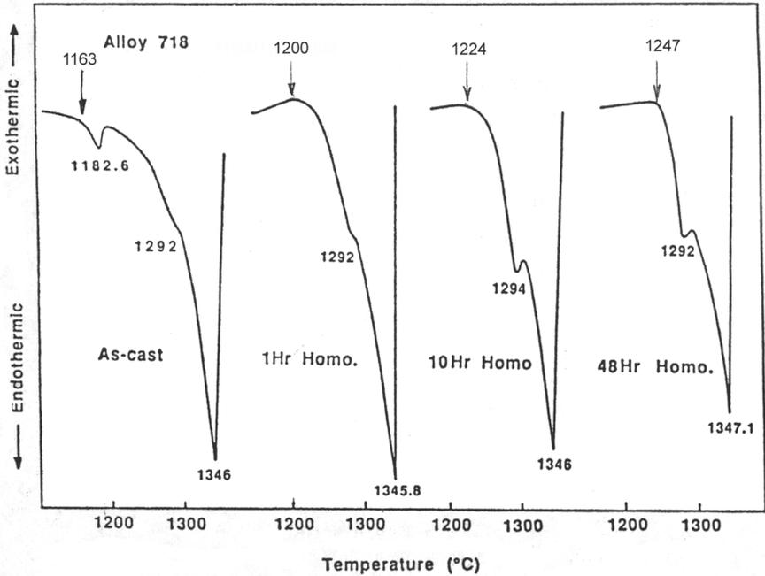
**Figure 3.7.** DTA signal for Inconel 718 showing the effect of annealing time [91Cao]. With annealing, the  $(Fe,Cr)_2Nb$  Laves phase dissolves and the onset of melting increases from 1163°C to 1247°C.
