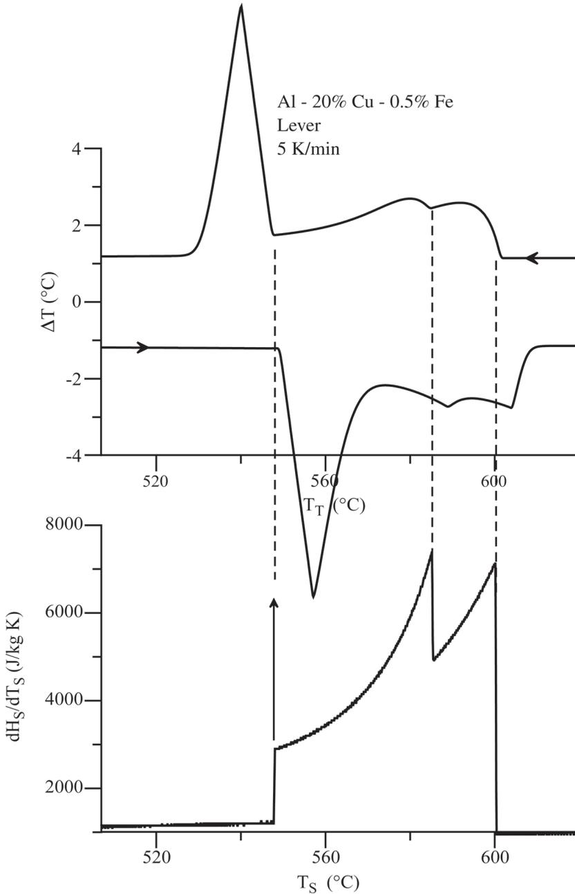
**Figure 4.2.** DTA and  $dH_S/dT_S$  plots for Al - 20 % Cu - 0.5 % Fe under equilibrium conditions. The aluminum alloy thermodynamic database [96Sau1] was employed. The solidification sequence is:  $L \rightarrow FCC$ ,  $L \rightarrow FCC + Al_7Cu_2Fe$ ,  $L \rightarrow FCC + Al_7Cu_2Fe + Al_2Cu$ .
