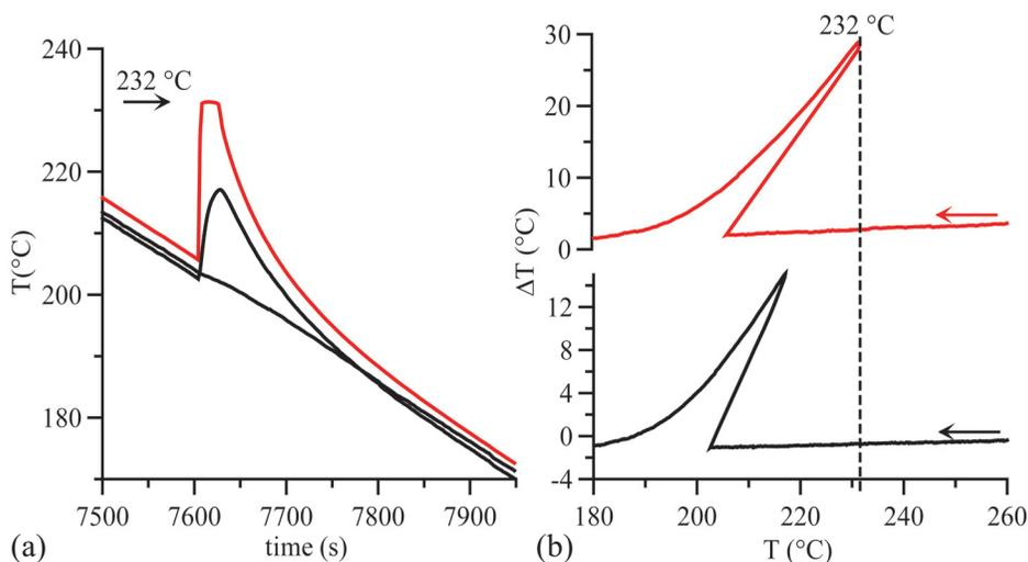
**Figure 3.15.** Measured (a) temperature vs. time plots and (b) associated DTA plots for the freezing of pure Sn. The instrument thermocouple readings (sample and reference) are black and the readings from a thermocouple immersed directly into the Sn in the sample cup are red. Significant supercooling has occurred prior to freezing inducing the rapid temperature rise upon solidification in (a) and the associated positive slope in (b); mass = 163.2 mg; heating rate = 5 K/min.
