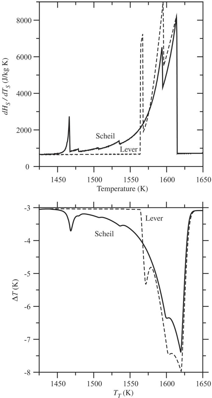
**Figure G5.** Top)  $dH_S/dT_S$  obtained from the enthalpy-temperature predictions for Udimet 700 alloy computed using thermodynamic database [96Sau2] for lever and Scheil conditions for Udimet 700 alloy. Bottom) Corresponding DTA plots for melting of 180 mg sample at 15 K/min.
