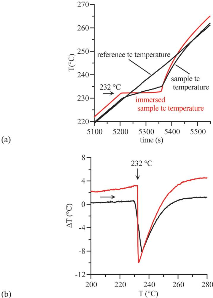
**Figure 2.6.** Measured (a) temperature vs. time plots and (b) associated DTA plots for melting of pure Sn. The instrument thermocouple readings are black and the readings from a thermocouple immersed directly in the Sn in the sample cup is red. Mass = 163.2 mg; heating rate = 5 K/min.
