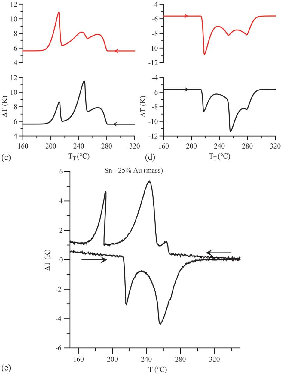
**Figure 3.17.** a) Phase diagram for Sn-rich alloys, b)  $H_S$  and  $dH_S/dT_S$  curves for Sn- 25 % Au calculated for equilibrium (black) and Scheil (red) conditions using the thermodynamic description of [03Liu]. Computed DTA curves for c) freezing and d) melting. Note how the amplitude of the peak for the “peritectic” reaction near  $252^{\circ}\text{C}$  is much reduced when the Scheil enthalpy is used. e) Experimental melting and freezing curves at 5 K/min.
