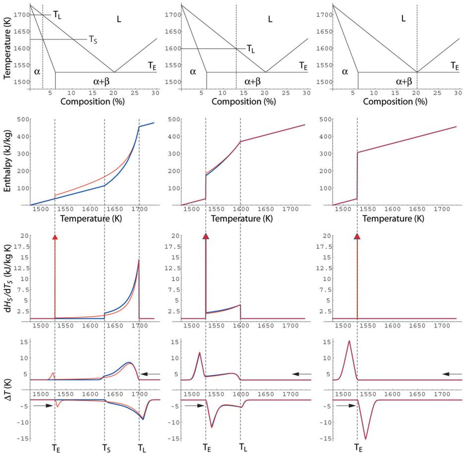
**Figure F1.** Phase diagram, enthalpy,  $dH_S/dT_S$  and computed DTA curves for three different compositions in a hypothetical binary eutectic system. The blue curves are for equilibrium conditions (Lever) and the red curves are for Scheil conditions.
