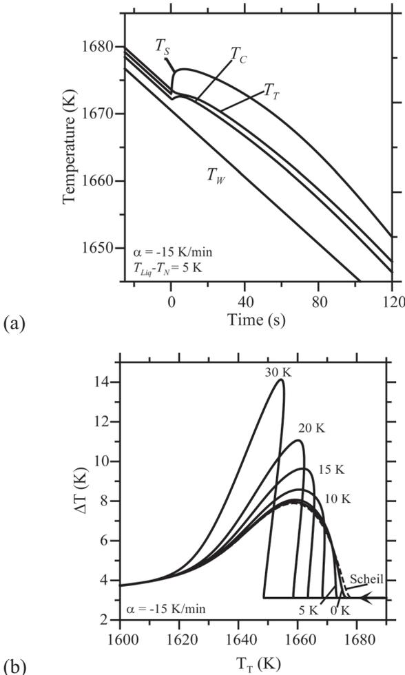
**Figure 3.16.** a) Plot of calculated sample, sample cup, sample thermocouple and furnace wall temperatures vs. time curves for dendritic freezing of a 180 mg sample of alloy with  $C_0 = 5\%$  at 15 K/min with an initial supercooling of 5 K/min. b) Effect of supercooling on the freezing DTA signal of the same alloy. The curves are for 0 K, 5 K, 10 K, 15 K, 20 K, 30 K supercooling. From [02Boe].
