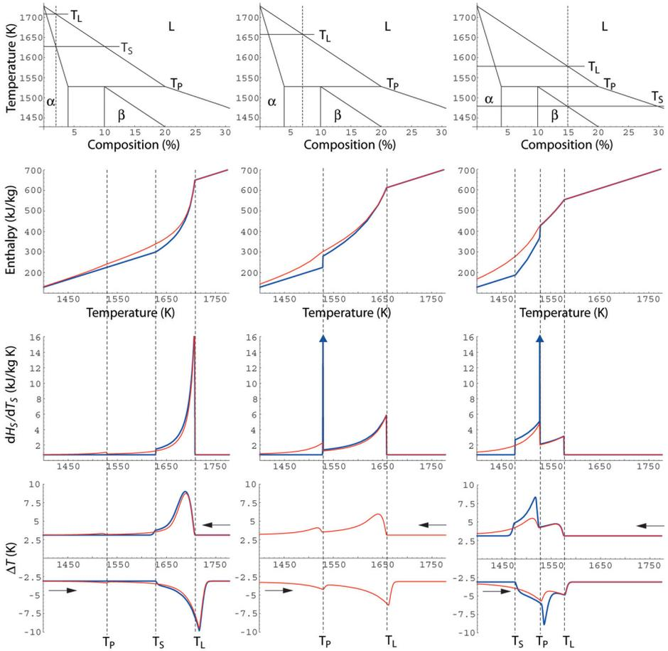
**Figure F2.** Phase diagram, enthalpy,  $dH_S/dT_S$  and computed DTA curves for three different compositions in a hypothetical binary peritectic system. The blue curves are for equilibrium conditions (Lever) and the red curves are for Scheil conditions.
