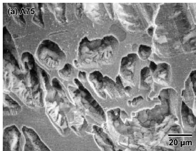
Fig. 9—Scanning electron micrograph of the fracture surface on alloy A75 in nitrogen gas at 50 °C.
