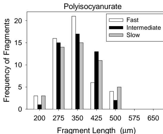
**Figure 4:** Distribution of fragment lengths in the isocyanurate samples tested with the three protocols.
