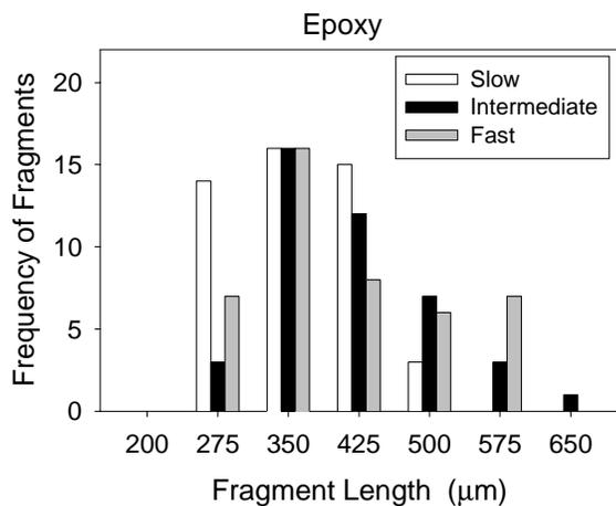
**Figure 3:** Distribution of fragment lengths for typical epoxy samples tested using the three protocols.
