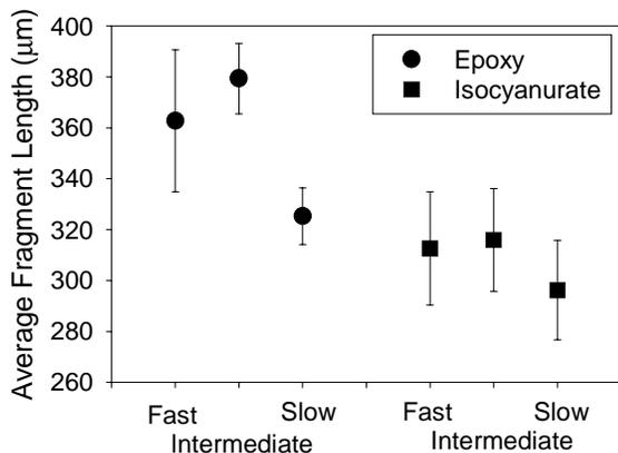
**Figure 2:** Average fragment length at saturation for the six sample-protocol combinations.
