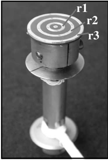
FIG. 2. Test fixture. The surface of the shearing disk consists of alternating nonconductive (polyimide) and conductive (aluminum) electrode rings ( r_1 , r_2 , and r_3 ) to improve accuracy of the shear-rate measurement.
