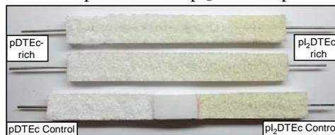
Fig. 2. Rod-shaped pDTEc/pI<sub>2</sub>DTEc scaffold libraries are at top of image. Control pDTEc (left) and pI<sub>2</sub>DTEc (right) scaffolds are at bottom. Stainless steel wires were incorporated into the scaffolds for reinforcement and to ease handling. Gradients range from 5 % to 83 % pDTEc by mass.
