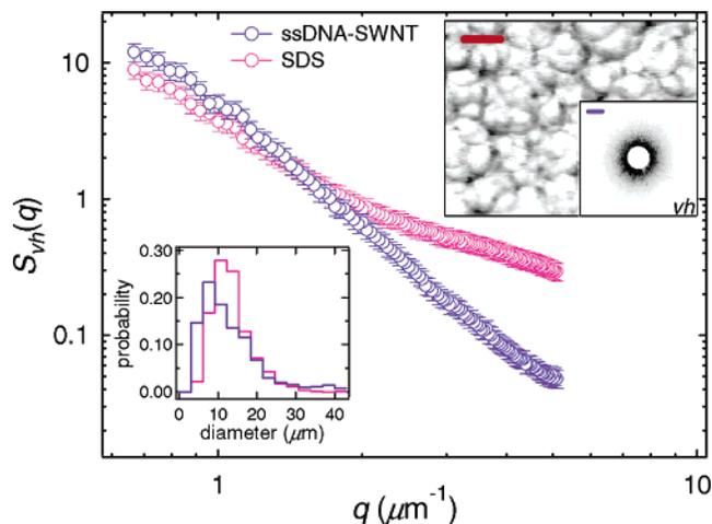
**Figure 4.** Cross-polarized small-angle light scattering profiles from the SWNT-stabilized and SDS-stabilized colloids saturated with Triton x100, where the upper right inset shows an optical micrograph/light-scattering pair for the SWNT coated particles (red scale bar = 60  $\mu\text{m}$ , purple scale bar = 1  $\mu\text{m}^{-1}$ ). The lower left inset shows diameter histograms for the two colloid types.
