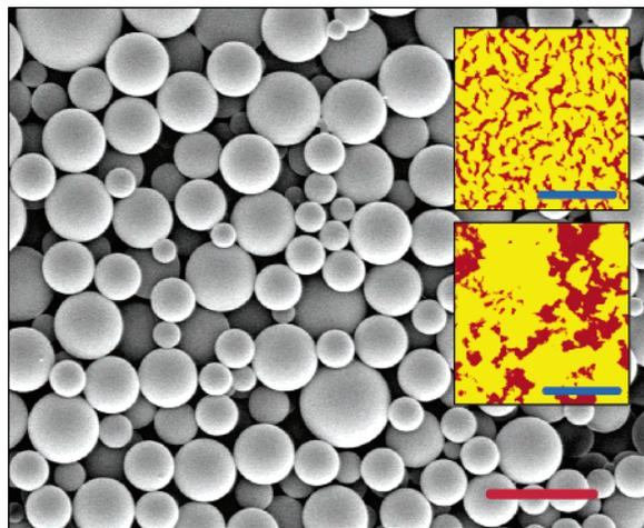
**Figure 3.** SEM image of dried SWNT-stabilized colloids (scale bar = 100  $\mu\text{m}$ ), where the upper inset shows an AFM image of a colloid surface and the lower inset shows an analogous image for an SDS stabilized colloid (phase contrast, scale bar = 150 nm).
