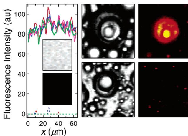
**Figure 5.** NIR fluorescence emission as a function of position for a dilute SWNT-ssDNA suspension, where the different colors represent measurements taken at 20 s intervals. The lower traces show the background emission intensity. This difference is shown visually in the inset. On the right, the upper two images show bright field (left) and NIR fluorescence (right) micrographs of stacked SWNT-stabilized colloids, whereas the lower images show the same for SDS-stabilized colloids.
