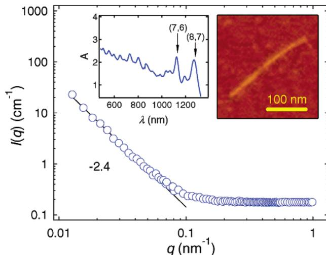
**Figure 1.** Typical SANS profile of the SWNT-ssDNA suspensions of interest here. The upper left inset shows the corresponding UV-vis absorption spectrum and the upper right inset shows an AFM image of an isolated ssDNA-coated SWNT deposited on a silicon wafer. The chirality vectors of the enriched semiconducting SWNT species are indicated. Unless otherwise indicated, error bars are the size of the data markers and represent two standard deviations in the total experimental uncertainty.
