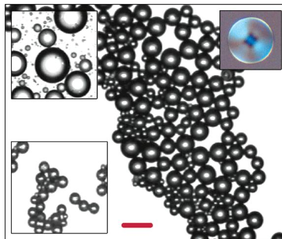
**Figure 2.** Optical micrograph of dried SWNT-coated colloids made of cross-linked polymer, where the red scale bar represents 70  $\mu$ m. The upper left inset is an emulsion of toluene in water stabilized by the ssDNA-wrapped SWNTs and the upper right inset is a dried SWNT-coated colloid under cross polarizers. The lower left inset shows control colloids made with SDS.
