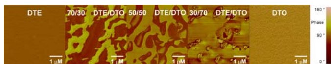
Figure 1. From left to right are five 5 μm × 5 μm AFM images in which the amount of DTO is increasing. The discrete DTE/DTO blends form phase-separated domains under in vacuo , 105 °C annealing conditions.
