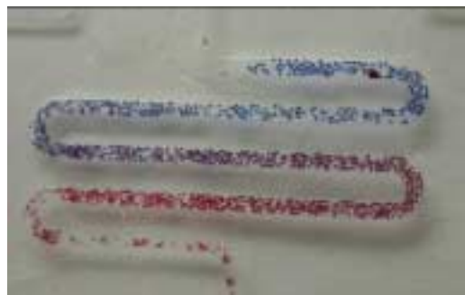
Figure 2. A collection of monomer droplets (approximately 300 μm in diameter) inside of a microfluidic channel. A gradient of composition is shown with benzyl methacrylate (dyed blue) and hexanediol dimethacrylate (dyed red).
