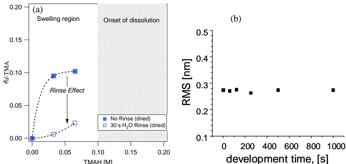
**Figure 6.** (a) Quantification of residual base trapped within ultrathin films. (b) Surface root-mean square (RMS) roughness of PNBHFA films immersed in 0.065 M developer as a function of time followed by a 60s water rinse.
