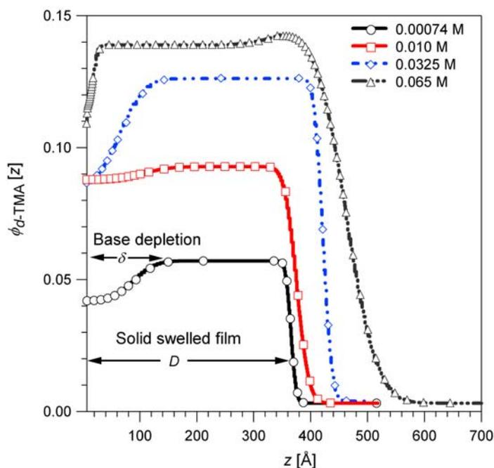
**Figure 3.** *d*-TMA counterion profiles within polyelectrolyte films versus distance from the silicon substrate with depleted level at the substrate and interfacial broadening at the solid / liquid interface.
