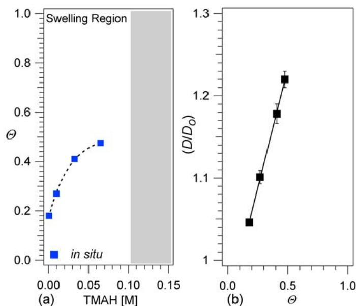
**Figure 4.** (a) Degree of polymer segment ionization ( $\Theta$ ) versus base concentration illustrating the lower limit of weak polyelectrolyte ionization before dissolution occurring above 0.10 M. (b) Expansion extent dependence on the calculated degree of ionization.
