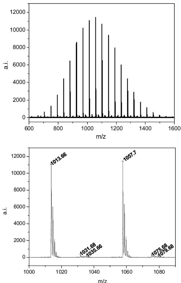
**Figure 3.** MALDI-TOF MS of 1k PEGDM, (a) full spectra and (b) expansion showing one main set of peaks 44 u apart due to Na<sup>+</sup> cationized PEGDM and two minor sets of peaks of PEGDM cationized by K<sup>+</sup> and H<sup>+</sup>, respectively.
