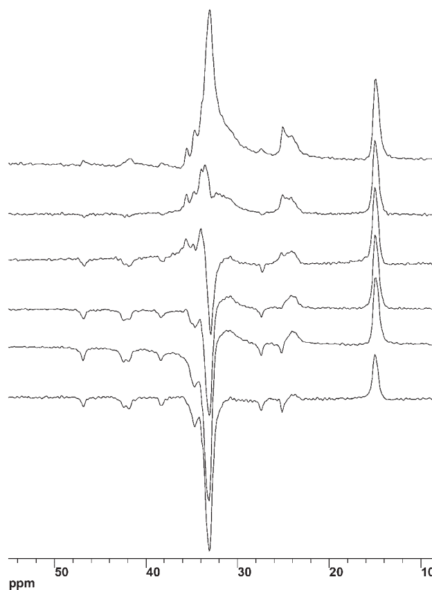
Figure 8. Distinguishing of rigid methylene and methine signals using polarization/depolarization spectra for the insoluble fraction (IF). After 5 ms of spin locking followed by 1 ms of cross polarization, there is a 180^\circ phase shift of the carbon rf for a duration of \tau_{ph} . Spectra from top to bottom have \tau_{ph} = 20, 23.2, 26.5, 30, 34 and 40 \mu\text{s} . Relatively rigid methylene carbons null near 23 \mu\text{s} , whereas methine carbons null near 35 \mu\text{s} . Motional averaging, e.g. for methyls near 15 ppm, increases the time needed for nulling.
