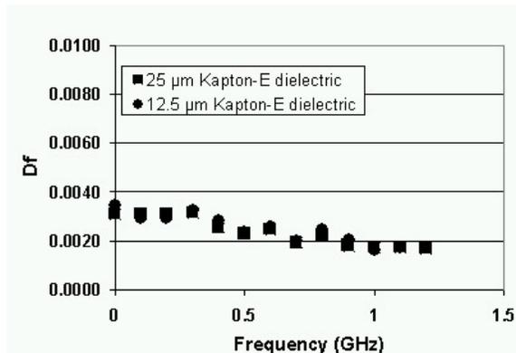
**Figure 2 - Dissipation Factor of T-foil**
