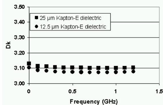
**Figure 1 - Dielectric Constant of T-foil**
