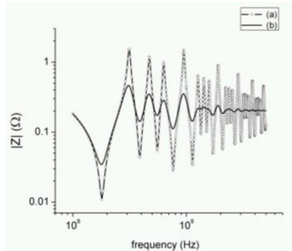
**Figure 6 - Input impedance calculated for 5 cm x 8 cm, 100  $\mu\text{m}$  thick power planes,  $D_k=38$ , (a)  $\tan(\delta) = 0.015$ , (b)  $\tan(\delta) = 0.15$**
