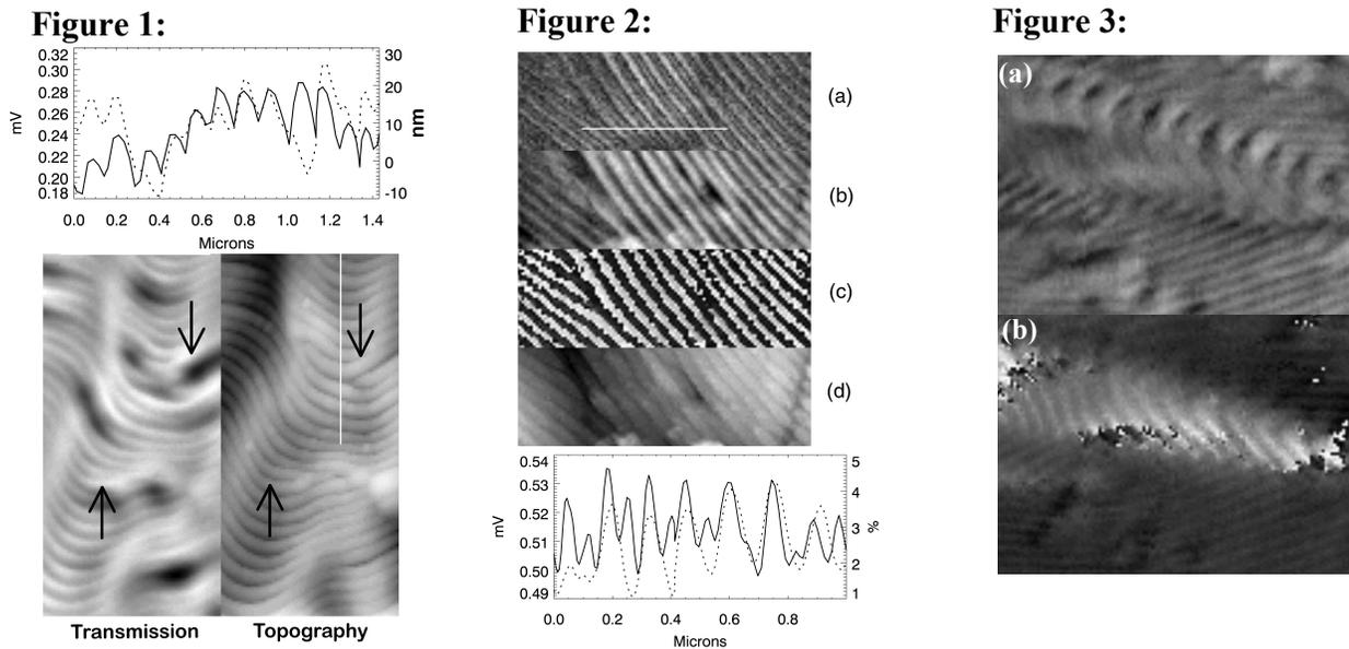
Fig. 1. NSOM micrograph of PS-b-PI. The top plot shows topography (dotted) and transmission (solid) along the white line (1.4  $\mu\text{m}$ ) in the topography image. Arrows indicate edge defects.
