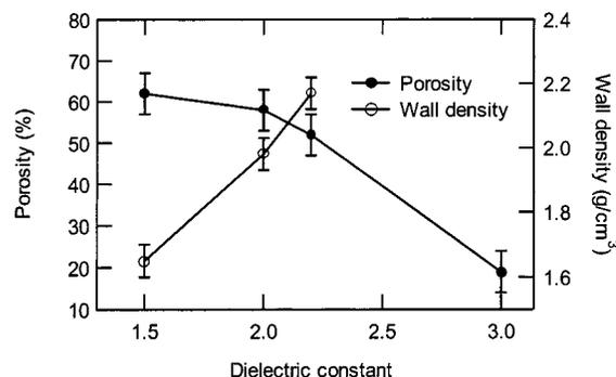
**Figure 7.** Porosity and wall density shown as a function of the dielectric constant. The  $k$  value from a standard HSQ is also shown for comparison. The solid lines are solely intended to emphasize trends in the experimental data.
