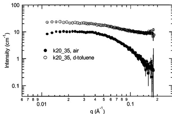
**Figure 5.** SANS data of the film with a dielectric constant of 2.0 and a Si-H fraction of 35% under ambient air conditions (filled symbols) and immersed in deuterated toluene (open symbols). Some error bars at the low  $q$  ranges are within the symbols.
