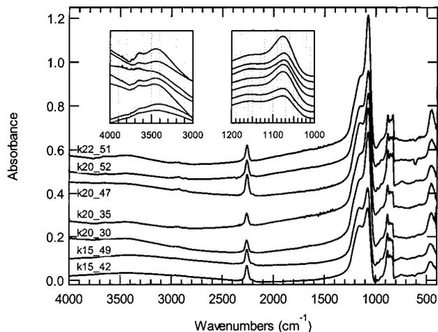
**Figure 8.** FTIR spectra of HSQ-based porous thin films with different process conditions presented as the relative intensity of absorbance versus wavenumber. The inset shows clearly the differences of the Si–O stretching peak position in the range of 1000–1200  $\text{cm}^{-1}$  and Si–OH peaks in the range of 3000–4000  $\text{cm}^{-1}$ . Curves are offset vertically for clarity.
