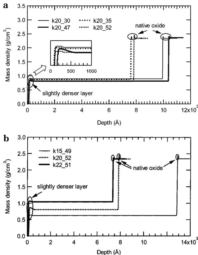
**Figure 4.** Electron density depth profiles of the films in Figure 3. a Films with a dielectric constant of 2.0 and different Si-H fractions of 30%, 35%, 47%, and 52%. The inset shows clearly the region of a slightly denser layer from the free surface to the depth of 1000 Å. b Films with a similar range of Si-H fractions ranging from 49% to 51% and different dielectric constants of 1.5, 2.0, and 2.2.
