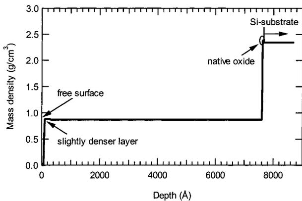
**Figure 2.** Calculated electron density depth profile of the film in Figure 1. The free surface is located at the far left of the horizontal axis, and the silicon substrate is located at the far right of the abscissa.
