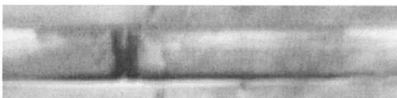
Classic epoxy system shows no interfacial damage near fiber breaks
