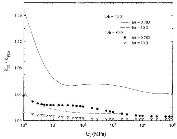
**Fig. 8 Comparison of the analytical stiffness based on Eq. (4),  $K_{s2}$ , to the stiffness ( $K_{FEA}$ ) from FEA under different aspect ratio  $L/h$**
