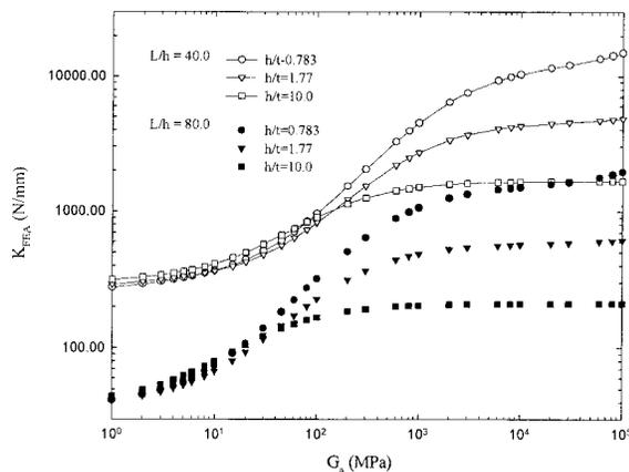
**Fig. 7 Beam stiffness from finite element analysis,  $K_{FEA}$ , as a function of adhesive shear modulus,  $G_a$ , for samples with 2 different span lengths,  $L$**
