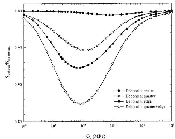
Fig. 11 The comparison of results between debonding and non-debonding with respect to adhesive shear modulus  $G_a$  ( $h/t = 0.783$ ,  $a/l = 0.1$ ,  $a$ : crack length)
