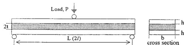
Fig. 1 The 3-point bending sandwich beam, the gray adhesive layer between two adherends
