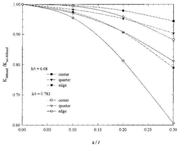
**Fig. 12 The comparison of results between debonding and no-debonding with respect to the length of debonds ( $G_a = 1.06$  GPa)**
