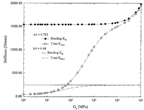
Fig. 4 The variation of the total stiffness and bending stiffness with respect to adhesive shear modulus
