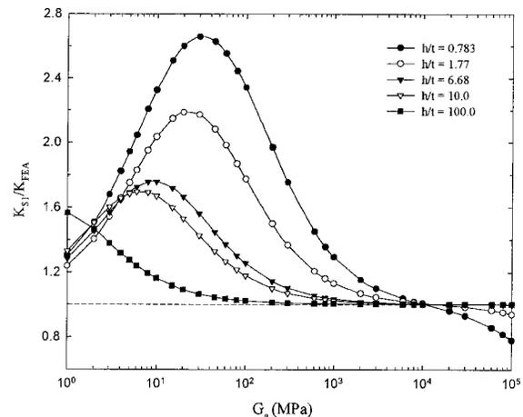
Fig. 5 Comparison of the analytical stiffness based on Eq. (1),  $K_{s1}$ , to the stiffness  $K_{FEA}$  from FEA
