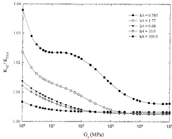
**Fig. 6 Comparison of the analytical stiffness based on Eq. (4),  $K_{s2}$ , to the stiffness  $K_{FEA}$  from FEA**
