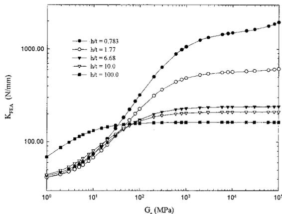
Fig. 3 The stiffness of the sandwich beam  $K_{FEA}$  obtained from the FEA
