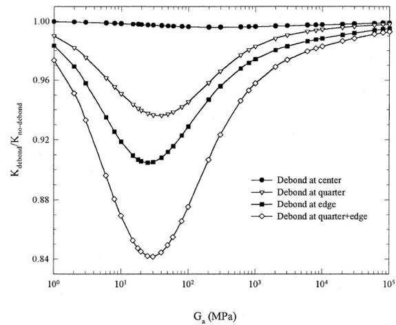
Fig. 10 The comparison of results between debonding and non-debonding with respect to adhesive shear modulus  $G_a$  ( $h/t = 6.68$ ,  $a/l = 0.1$ ,  $a$ : crack length)
