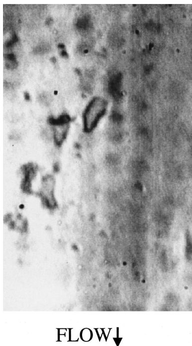
FIG. 7. Micrograph of several slow moving/stuck gel particles that are observed 1300 s after the addition of the fluoropolymer additive. The height of the micrograph corresponds to 200 \mu\text{m} .
