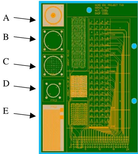
Fig. 1. Test patterns A-E for dielectric characterization of embedded capacitance films at DC and low frequencies
