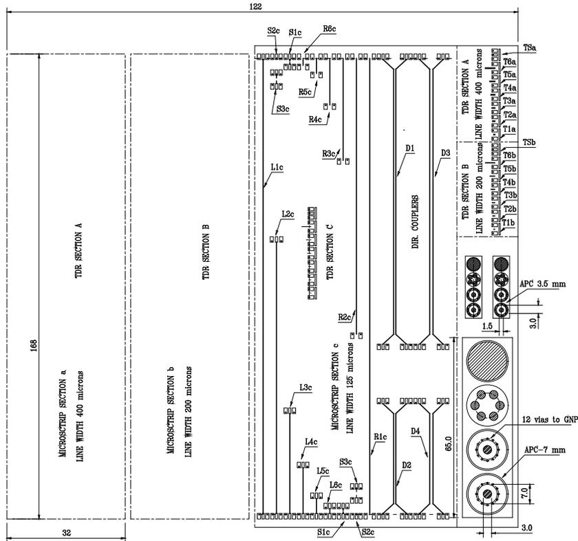
Fig.2 Schematic of the high frequency test vehicle
