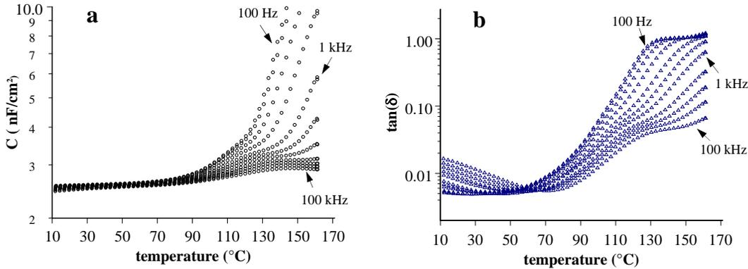
Fig.10. Capacitance density (a) and the dielectric loss tangent (b) of C-Ply as a function of temperature and frequency.(TV0 /3M, pattern B)
