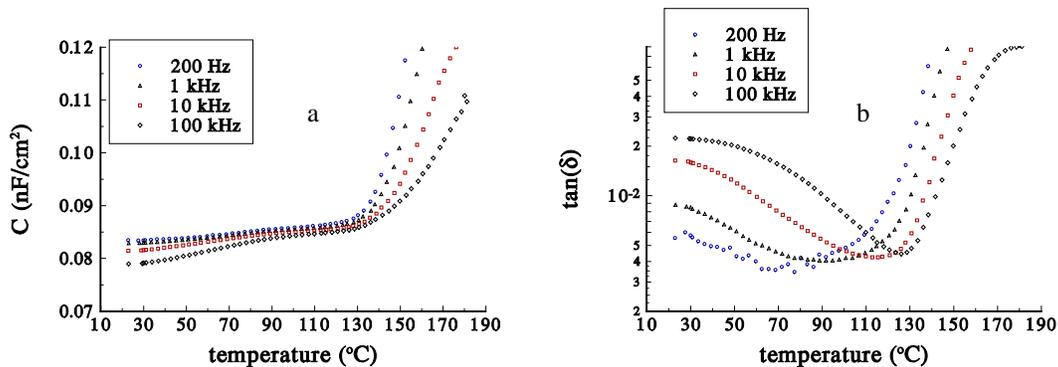
Fig.7. Capacitance density (a) and the dielectric loss tangent (b) of BC2000 as a function of temperature and frequency.(TV0 / HADCO, pattern B)
