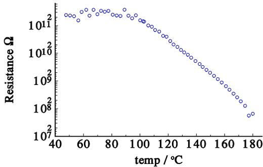
Fig.4. Insulation resistance of FR4 laminate under bias of 100V as a function of temperature
