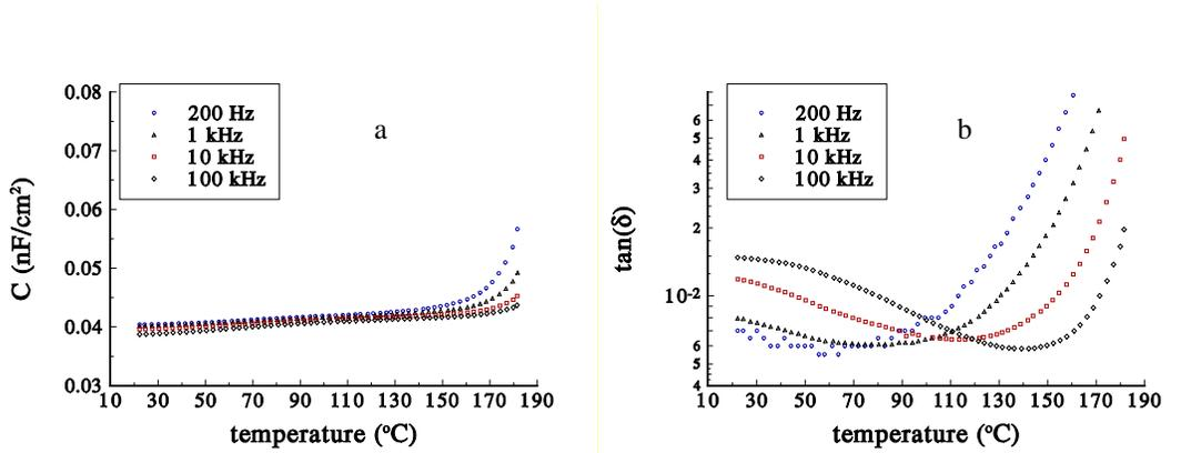
Fig.5. Capacitance density (a) and the dielectric loss tangent (b) of FR4 as a function of temperature and frequency.(TV0 / Merix, pattern B)
