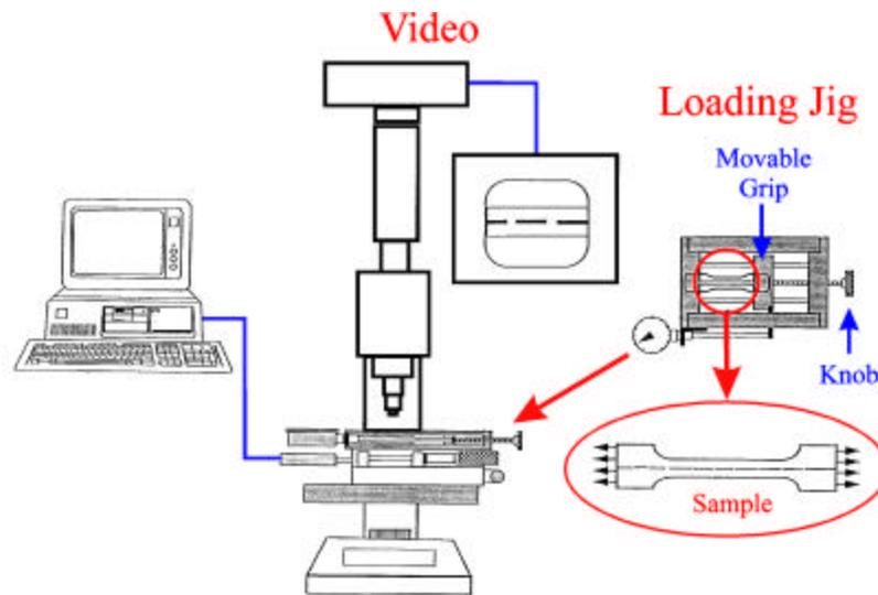
**Figure 1. Schematic of Testing Apparatus.**
