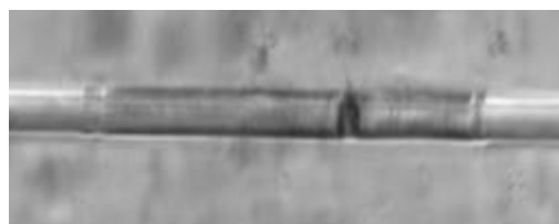
Figure 2: Failure zone at the fiber-matrix interface.
