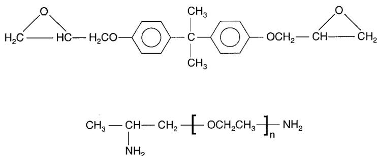
**FIG. 5.** The amine hardened epoxy resin system is shown above. The top structure is Tactix 123. The bottom structure is Jeffamine D400.
