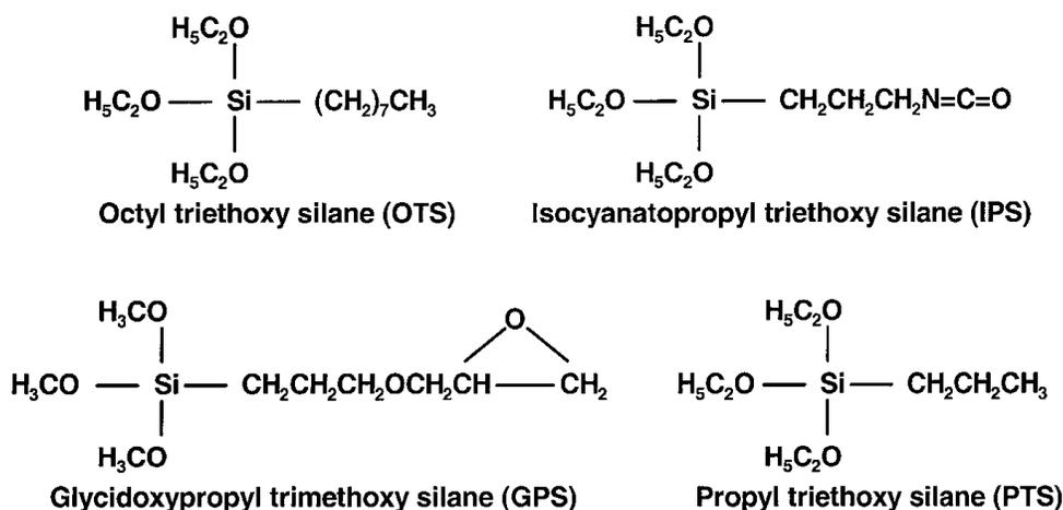
FIG. 2. Coupling agents used in the dilution of the DMSCA dye at the glass surface.
