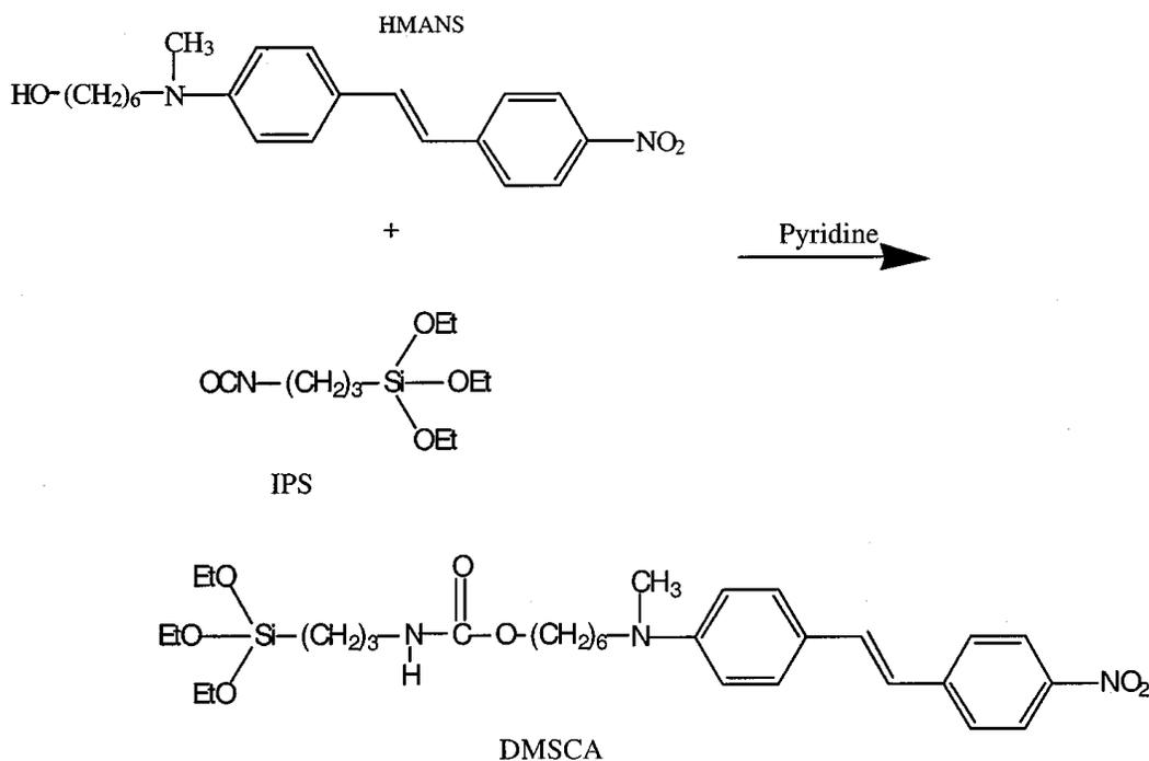
FIG. 3. A fluorescent dye is reacted with a triethoxy silane coupling agent to generate the DMSCA molecule.
