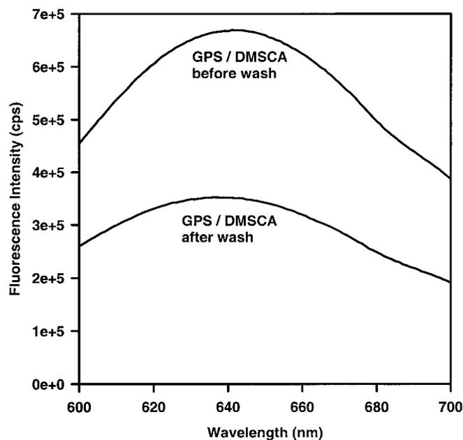
**FIG. 7.** A decrease in fluorescence intensity is observed from the grafted GPS/DMSCA layer after an acetone wash.
