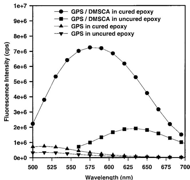
**FIG. 6.** A blue shift is observed from the grafted DMSCA dye during cure of an epoxy overlayer.
