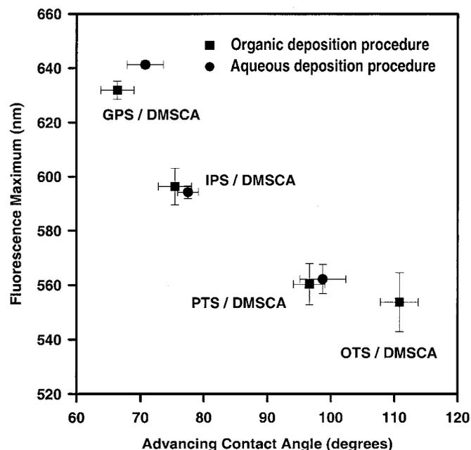
**FIG. 9.** Position of the fluorescence emission of the grafted DMSCA as a function of the layer surface energetics and the deposition procedure.
