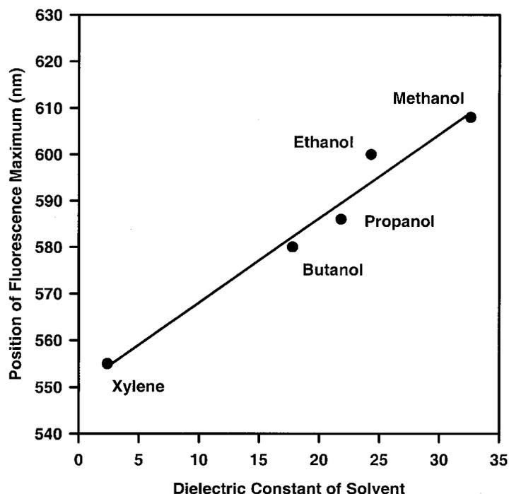
FIG. 11. Position of the fluorescence maximum from DMANS when dissolved in solvents of different polarity.
