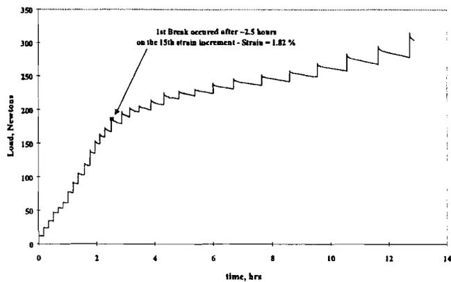
Fig. 1. Load-Time Curve of Bare E-Glass Fiber Specimen.
