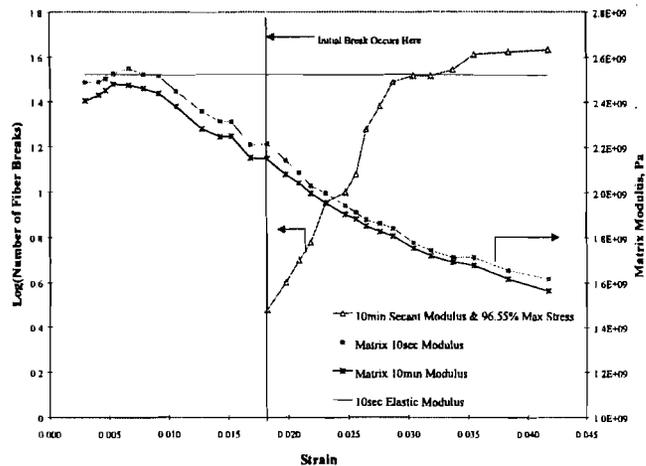
Fig. 2. Variation of Secant Modulus and Number of Fiber Breaks with Strain.
