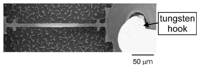
Fig. 6. SEM image of a specimen ready for testing with tungsten hook engaged in the loading hole.
